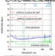
MEASURED ON MAXM17633 EV KIT WITH C =  $0.22 \mu F, \ L$  =  $22 \mu H$
