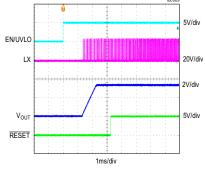
MAXM17633/MAXM17635 STARTUP THROUGH ENABLE  $V_{OUT}$  = 3.3V, f<sub>SW</sub> = 800kHz, 20mA LOAD, PFM MODE
