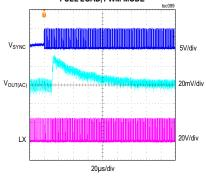
MAXM17634/MAXM17635 OUTPUT SHORT DURING STARTUP V<sub>OUT</sub> = 5V, f<sub>SW</sub> = 1MHz, FULL LOAD, PWM MODE
