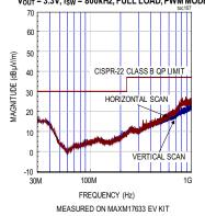
$\begin{array}{l} \text{MAXM17633/MAXM17635 CONDUCTED EMISSIONS PLOT} \\ V_{\text{OUT}} = 3.3 V, \, f_{\text{SW}} = 800 \text{kHz}, \, \text{FULL LOAD}, \text{PWM MODE} \end{array}$
