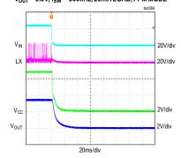
MAXM17634/MAXM17635 STARTUP THROUGH IN V<sub>OUT</sub> = 5V, f<sub>SW</sub> = 1MHz, FULL LOAD, PWM MODE
