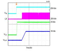
MAXM17635 STARTUP THROUGH IN V<sub>OUT</sub> = 2.5V, f<sub>SW</sub> = 700kHz, 20mA LOAD, PFM MODE
