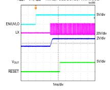
MAXM17634/MAXM17635 SHUTDOWN THROUGH IN  $V_{OUT}$  = 5V, f<sub>SW</sub> = 1MHz, 20mA LOAD, PFM MODE
