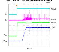
MAXM17634/MAXM17635 STARTUP THROUGH ENABLE (3.3V PREBIAS) V<sub>OUT</sub> = 5V, f<sub>SW</sub> = 1MHz, FULL LOAD, PWM MODE
