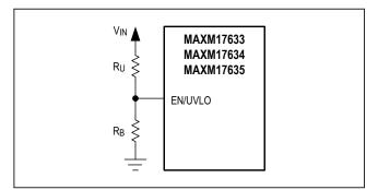
Figure 1. Setting the EN/UVLO Network
