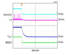
MAXM17633/MAXM17635 SHUTDOWN THROUGH ENABLE  $V_{\text{OUT}}$  = 3.3V,  $f_{\text{SW}}$  = 800kHz, FULL LOAD, PWM MODE
