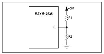
Figure 2. Setting the Output Voltage
