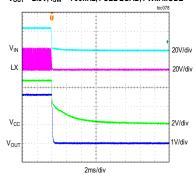
$\label{eq:maxm17633} \begin{array}{l} \mbox{MAXM17635} \ \mbox{STARTUP} \ \mbox{THROUGH} \ \mbox{IN} \\ \mbox{V}_{OUT} = 3.3 V, \ \mbox{f}_{SW} = 800 \ \mbox{Hz}, \ \mbox{FULL} \ \mbox{LOAD}, \ \mbox{PWM} \ \mbox{MODE} \end{array}$
