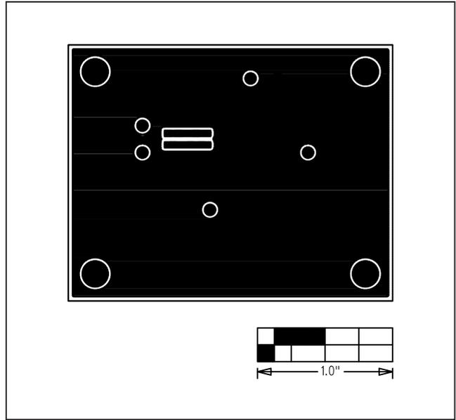
Figure 4. MAX9945 EV Kit PCB Layout—Solder Side
