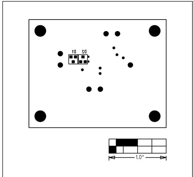
Figure 5. MAX9945 EV Kit Component Placement Guide—Solder Side
