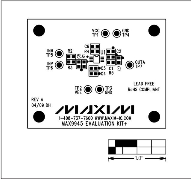
Figure 2. MAX9945 EV Kit Component Placement Guide—Component Side
