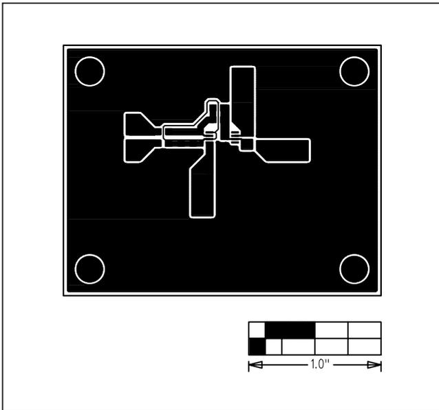
Figure 3. MAX9945 EV Kit PCB Layout—Component Side
