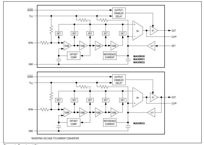
Figure 1. Functional Diagram
