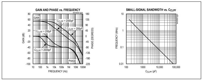
Figure 4. Gain and Phase vs. Frequency
