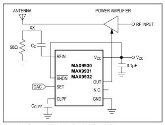
Figure 3. Control Mode Application Circuit Block
