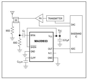
Figure 2. MAX9933 Typical Application Circuit
