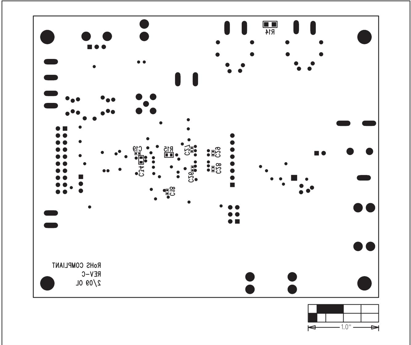
Figure 21. MAX9850 EV Kit Component Placement Guide—Solder Side
