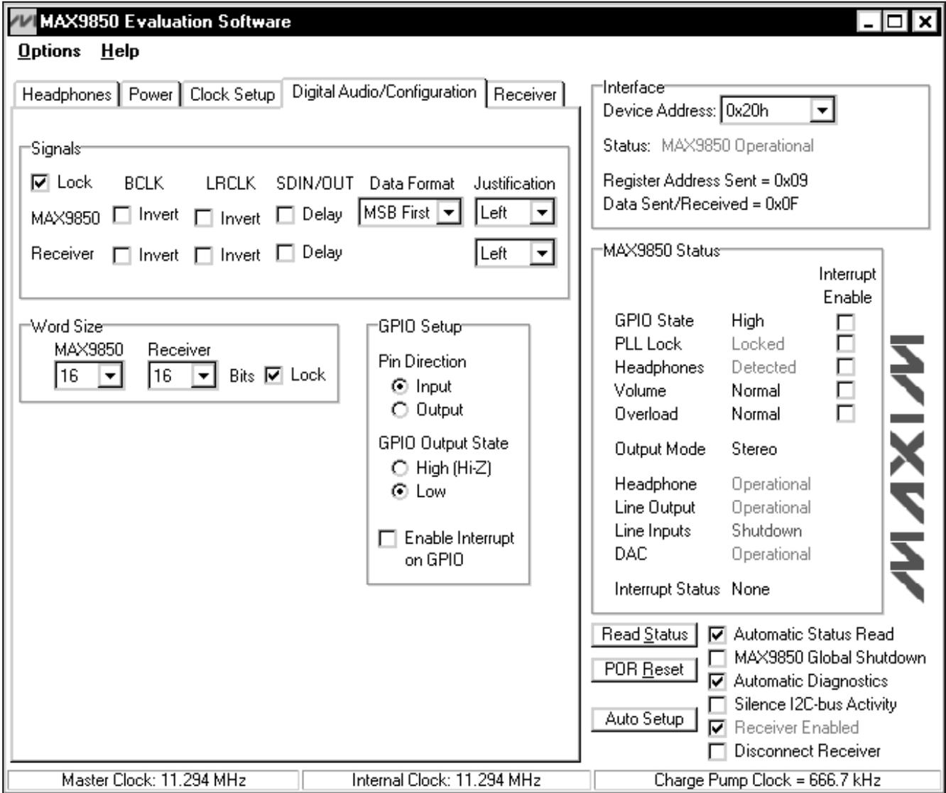
Figure 10. MAX9850 EV Kit Software Digital Audio/Configuration Tab
