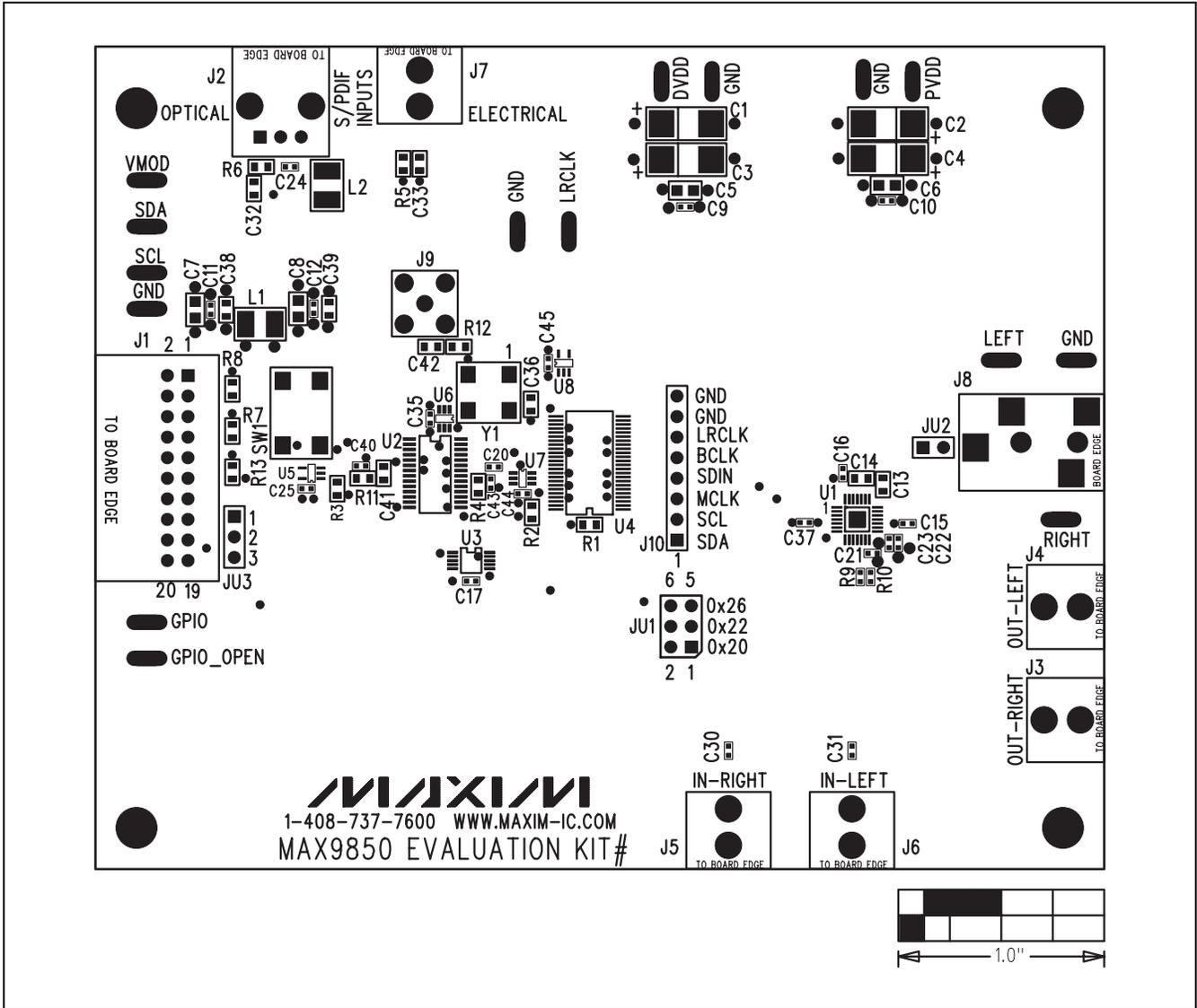
Figure 16. MAX9850 EV Kit Component Placement Guide—Component Side
