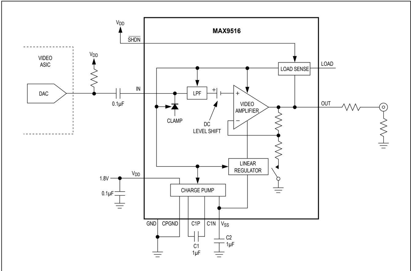
Figure 8. AC-Coupled Input
