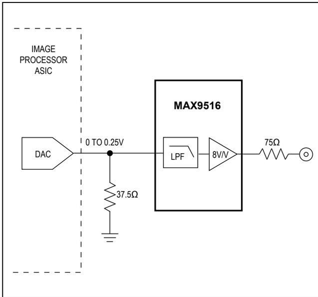
Figure 4. Video DAC Generates a 0.25V<sub>P-P</sub> Signal Across a 37.5Ω Resistor Connected to Ground
