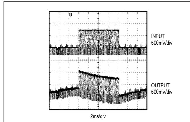
Figure 1. AC-Coupled Output
