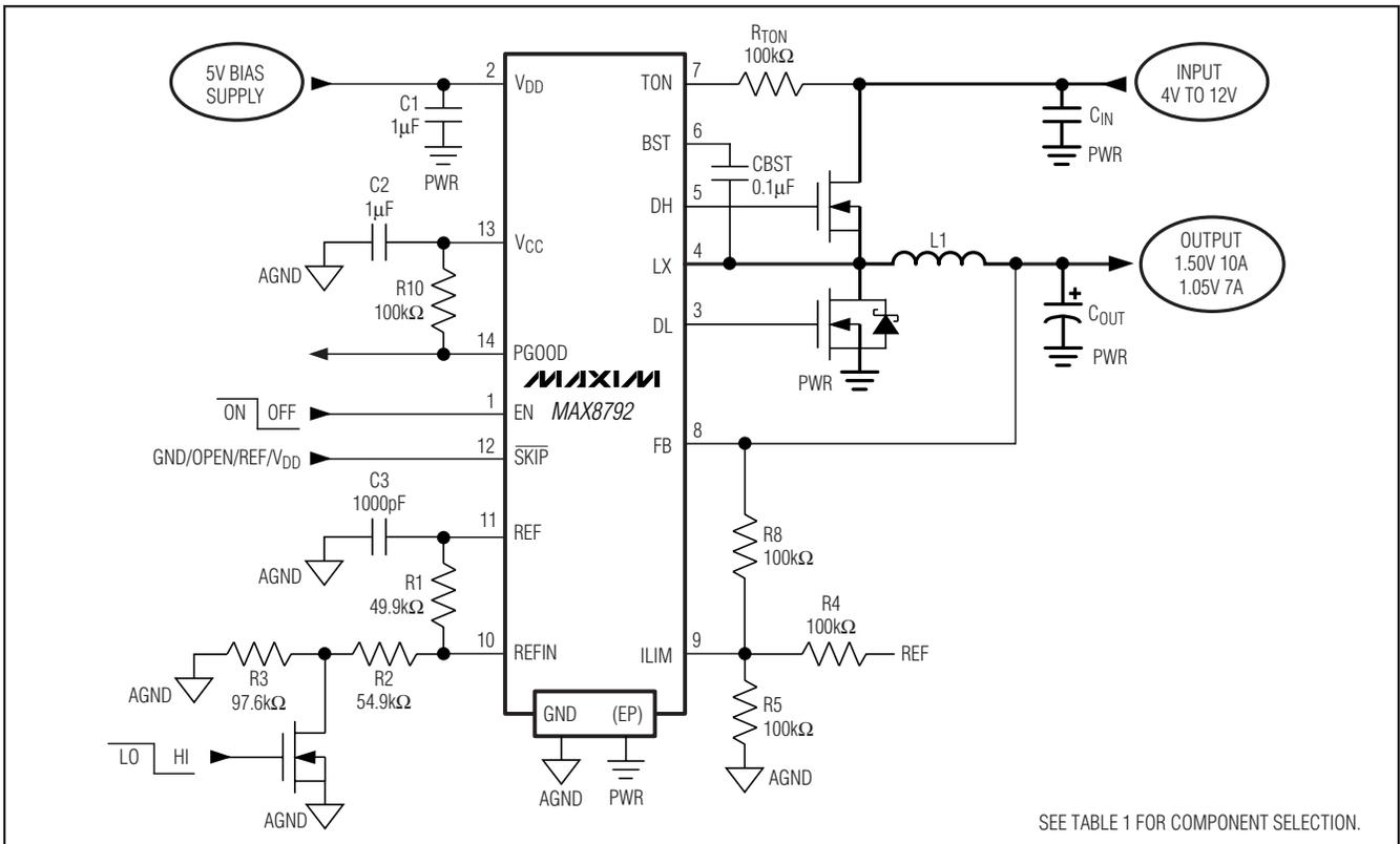
Figure 7. Standard Application with Foldback Current-Limit Protection
