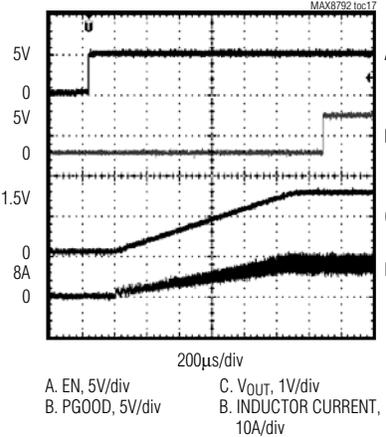
**SOFT-START WAVEFORM (LIGHT LOAD)**
