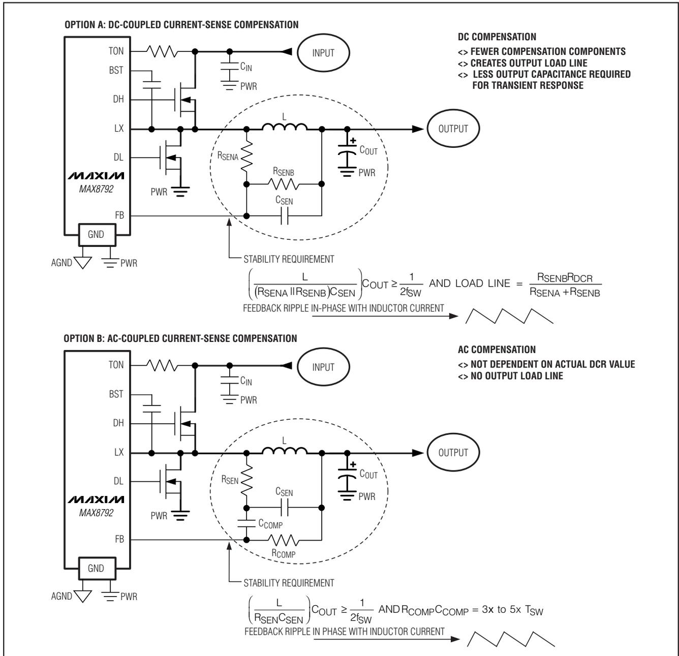
Figure 10. Feedback Compensation for Ceramic Output Capacitors
