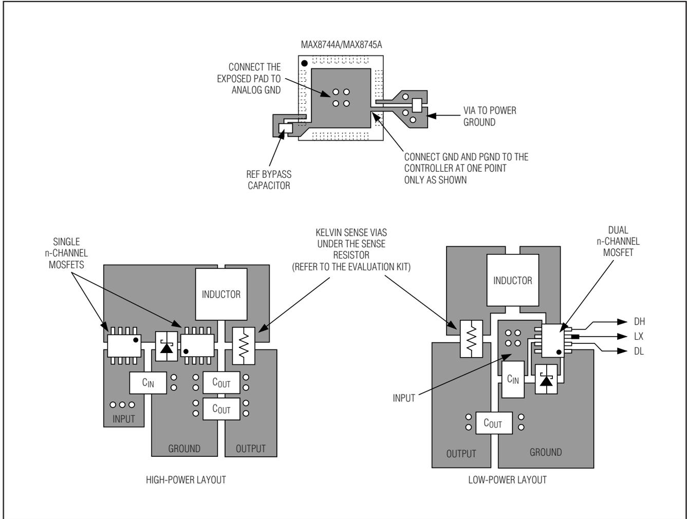
Figure 9. PCB Layout
