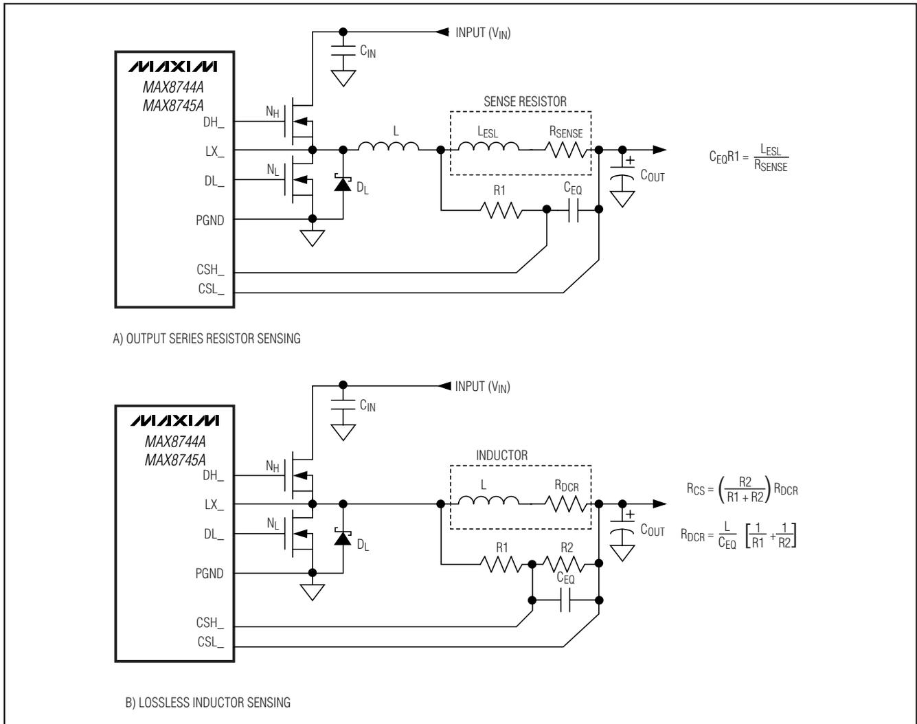
Figure 7. Current-Sense Configurations
