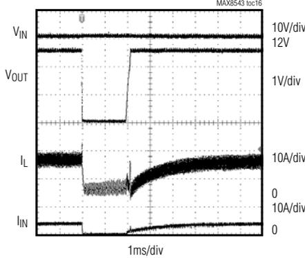
**OVERVOLTAGE PROTECTION WITH 15A LOAD**
