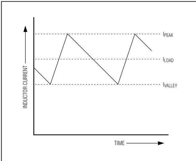
Figure 4. Inductor-Current Waveform
