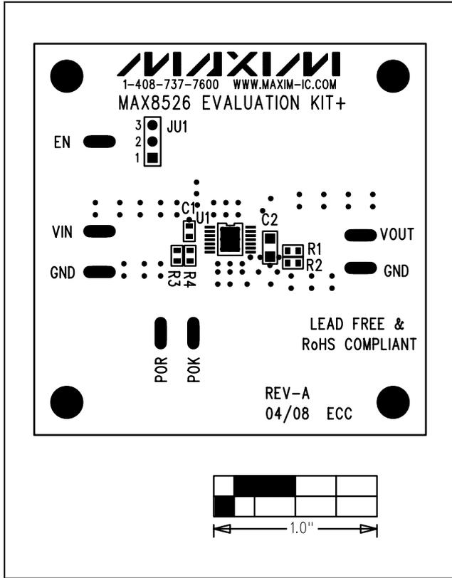
Figure 2. MAX8526 EV Kit Component Placement Guide—Component Side
