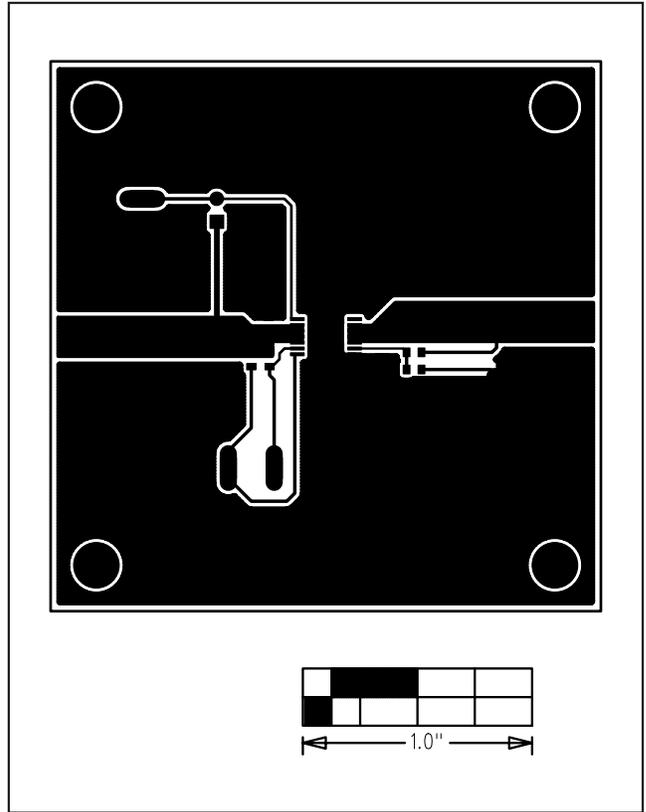
Figure 3. MAX8526 EV Kit PCB Layout—Component Side
