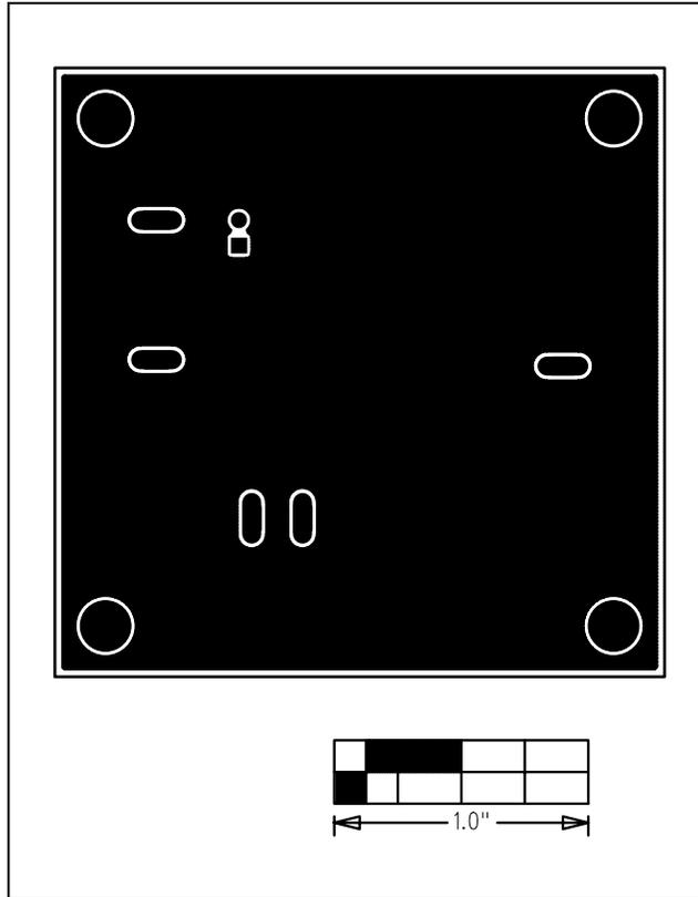
Figure 4. MAX8526 EV Kit PCB Layout—Solder Side
