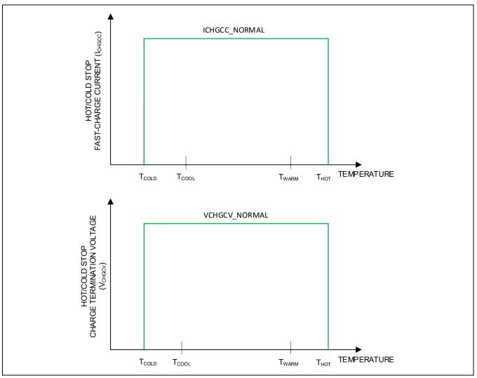
Figure 11. MAX77787H Version Hot/Cold Stop
