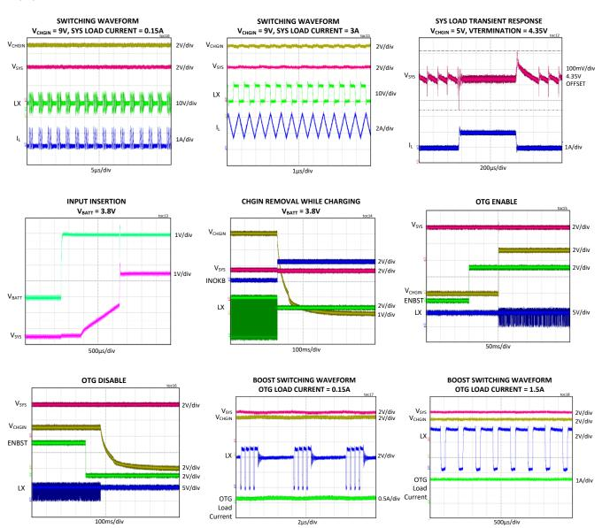
(V<sub>CHGIN</sub> = 5V, V<sub>BATT</sub> = 3.8V,  $T_A$  = +25°C, unless otherwise noted.)
