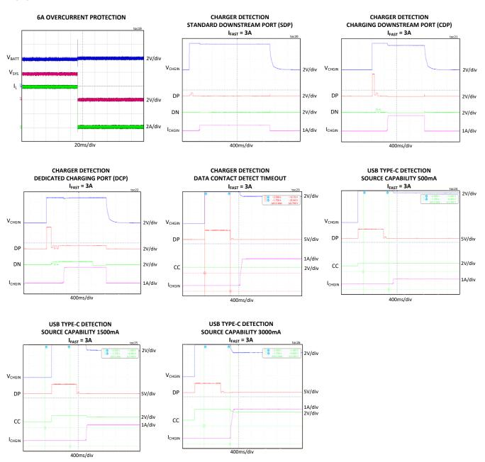
(V<sub>CHGIN</sub> = 5V, V<sub>BATT</sub> = 3.8V,  $T_A$  = +25°C, unless otherwise noted.)
