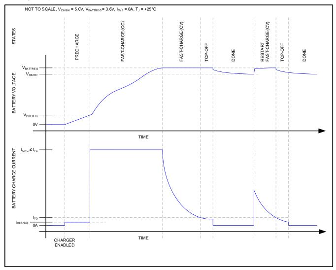
Figure 7. LiFePO<sub>4</sub> Battery Charge Profile
