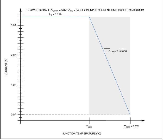
Figure 9. Charge Currents vs. Junction Temperature
