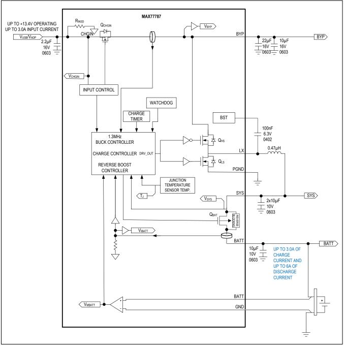
Figure 2. Main Battery Charger Detailed Functional Diagram
