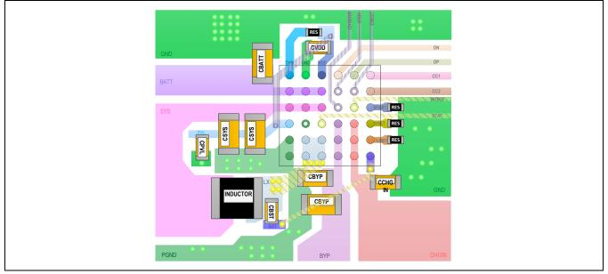
Figure 13. Recommended Placement and Layout
