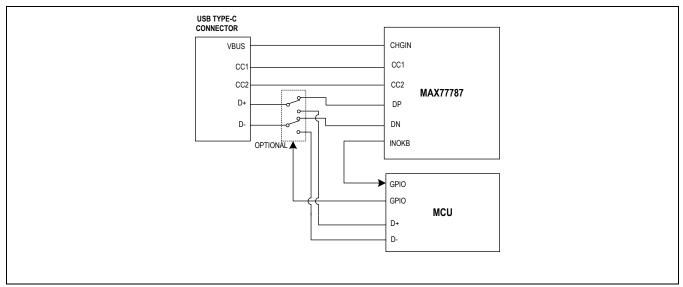
Figure 12. D+/D- Connections in a Reference System
