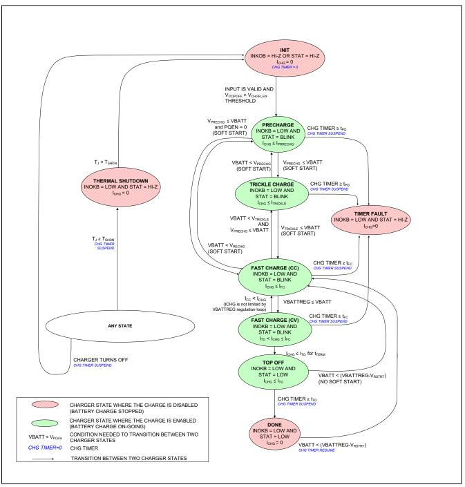
Figure 6. Li+/Li-Poly Charger State Diagram
