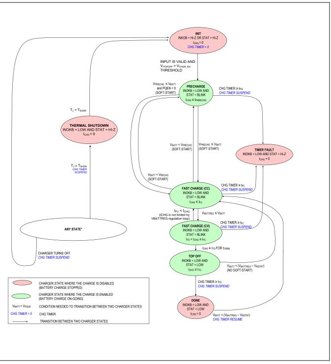
Figure 8. LiFePO<sub>4</sub> State Machine
