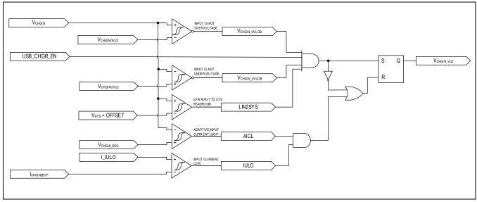
Figure 3. CHGIN Valid Signal Generation Logic
