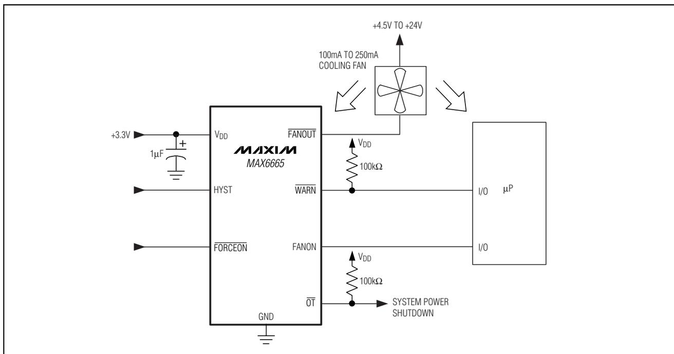
Figure 1. High-Reliability, Fail-Safe Fan Controller and Temperature Monitor
