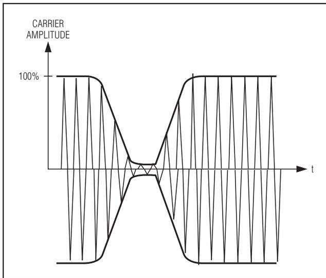
Figure 6. Downlink Modulation (e.g., Approximately 100% Amplitude Modulation)
