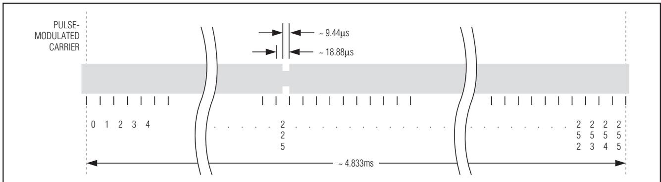
Figure 7. Downlink Data Coding (Case “1 Out of 256”)
