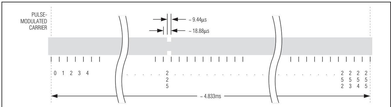
Figure 6. Downlink Data Coding (Case “1 Out of 256”)
