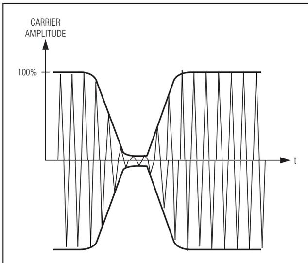
Figure 5. Downlink Modulation (e.g., Approximately 100% Amplitude Modulation)
