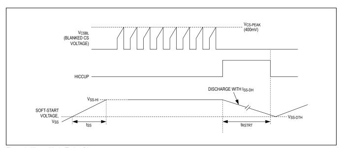
Figure 6. Hiccup Mode Timing Diagram
