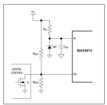
Figure 1. Programmable UVLO for the Power Source
