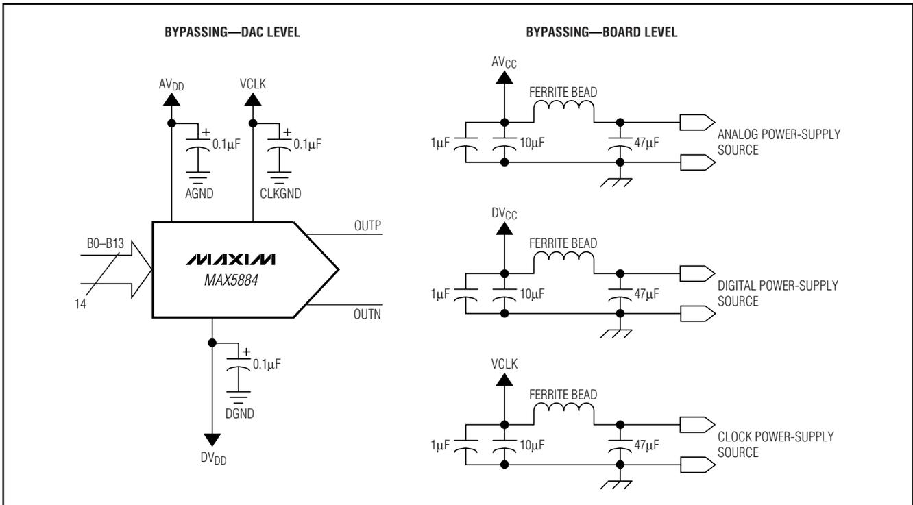
Figure 12. Recommended Power-Supply Decoupling and Bypassing Circuitry
