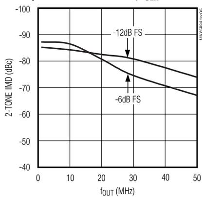
**2-TONE INTERMODULATION DISTORTION ( $f_{CLK} = 100MHz$ )**
