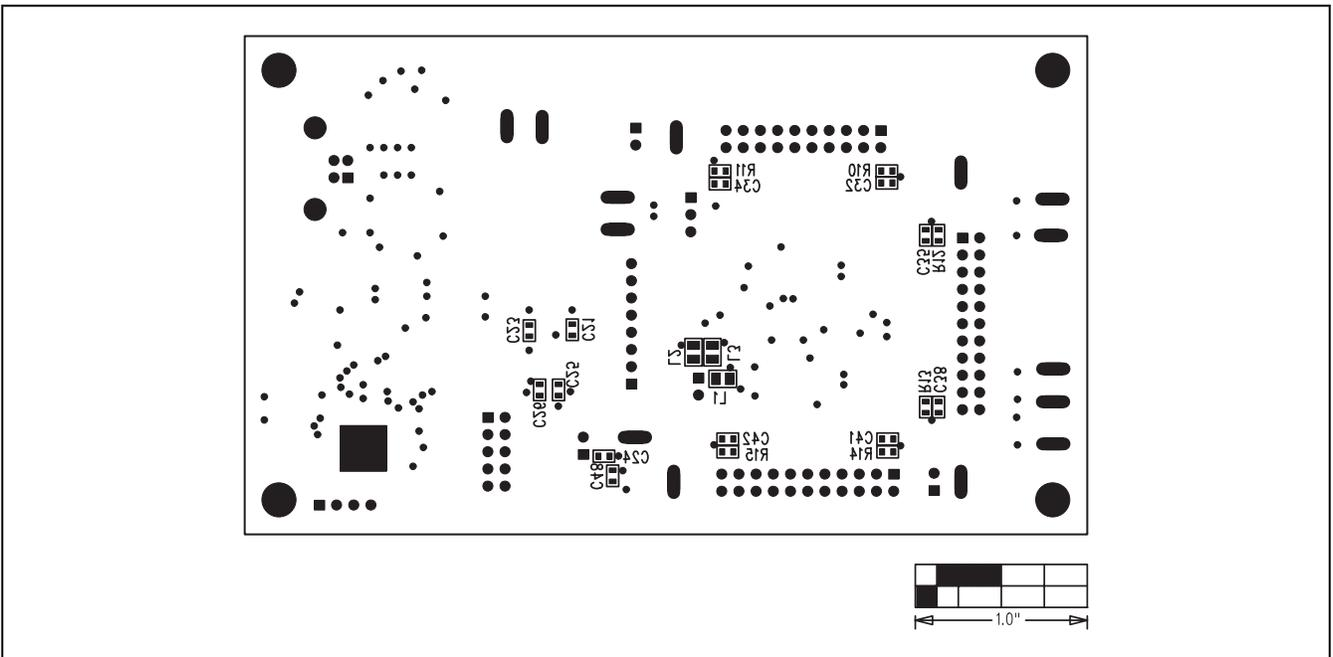
Figure 9. MAX5774 EV Kit Component Placement Guide—Solder Side
