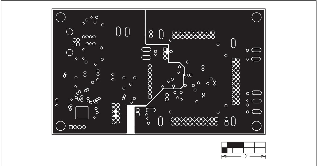
Figure 6. MAX5774 EV Kit PCB—Ground Planes (Layer 2)
