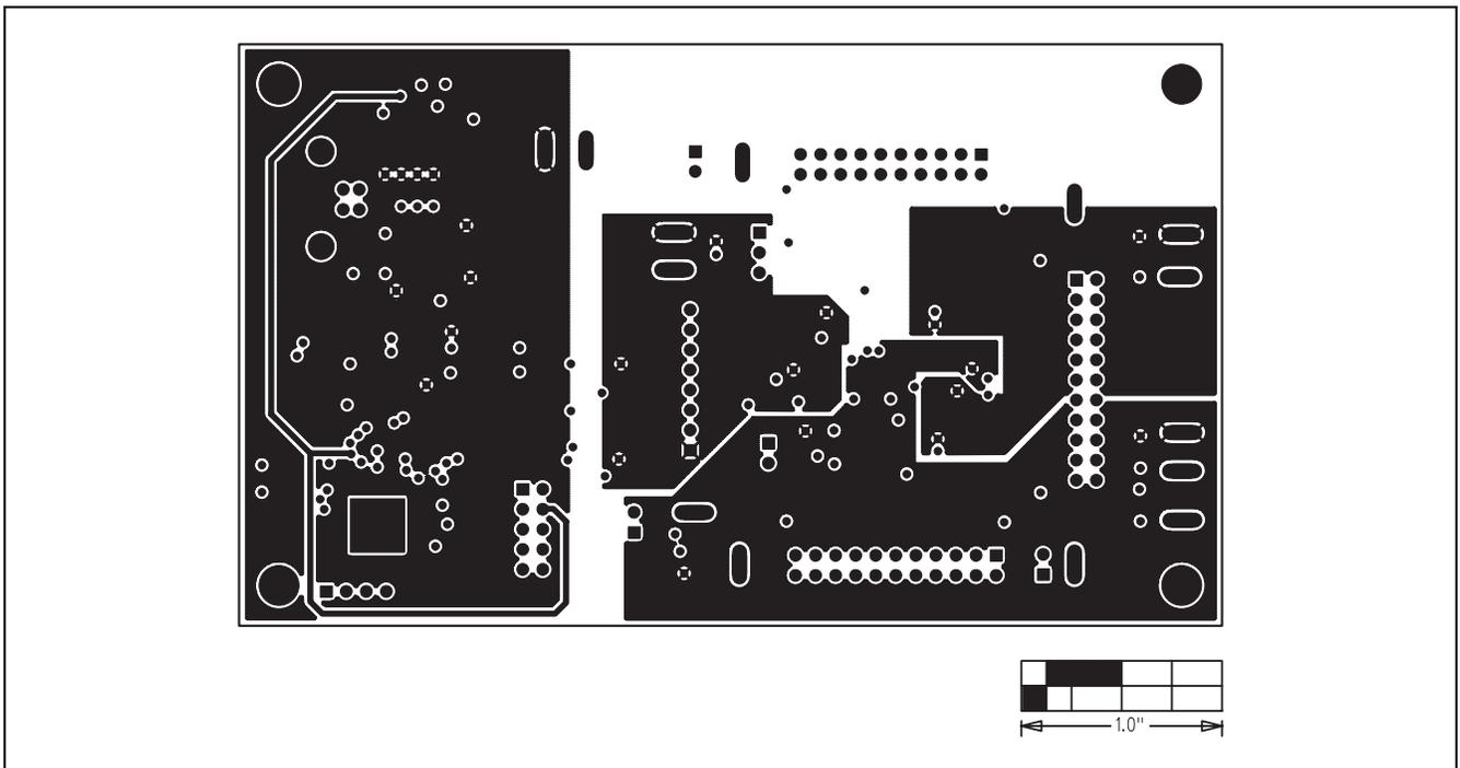
Figure 7. MAX5774 EV Kit PCB—Power Planes (Layer 3)
