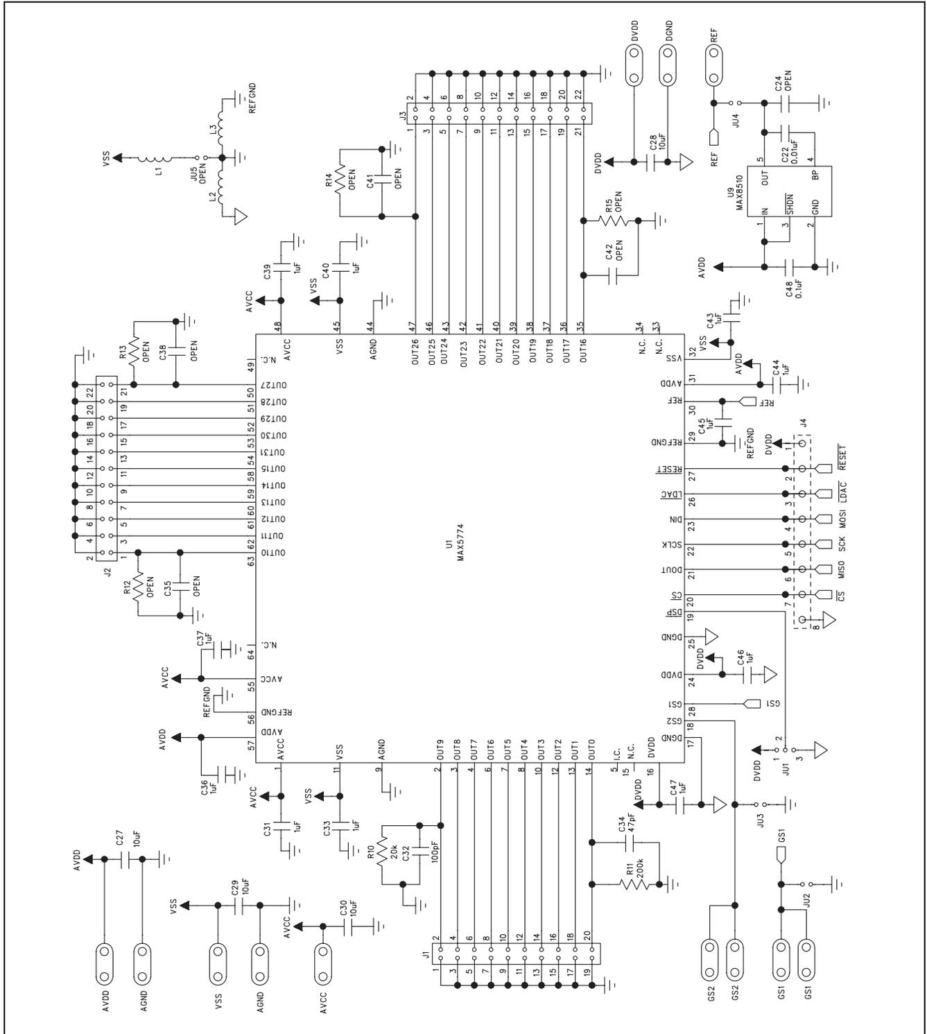
Figure 3a. MAX5774 EV Kit Schematic (Sheet 1 of 2)
