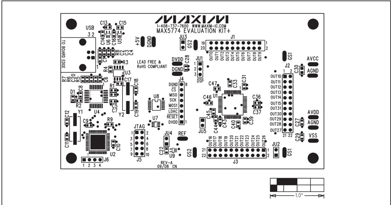
Figure 4. MAX5774 EV Kit Component Placement Guide—Component Side
