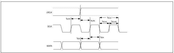
Figure 5. External SCLK Serial Timing Diagram
