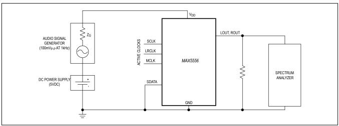
Figure 1. PSRR Test Block Diagram
