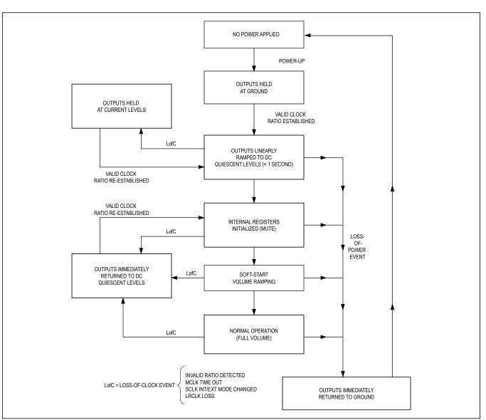
Figure 10. Internal State Diagram
