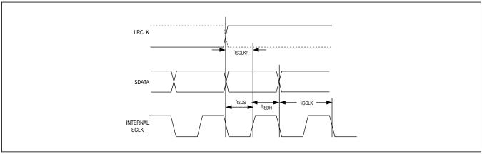
Figure 6. Internal SCLK Serial Timing Diagram
