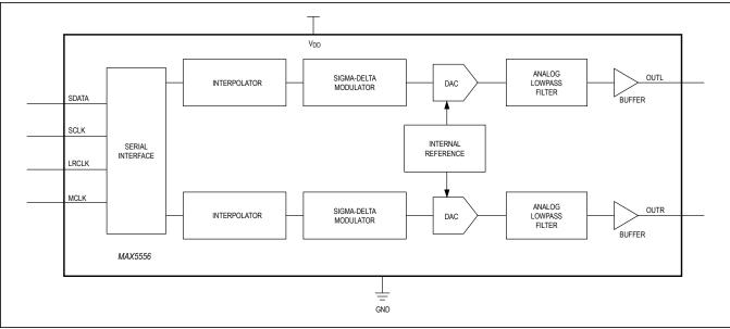
Figure 2. Functional Diagram
