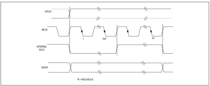
Figure 7. Internal Serial Clock Generation
