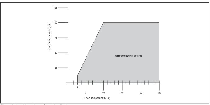
Figure 3. Load-Impedance Operating Region
