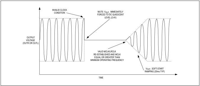
Figure 12. Invalid Clock Output Response
