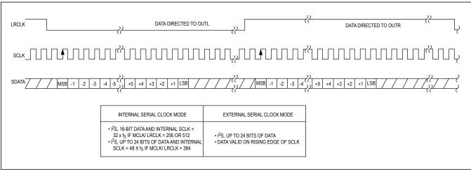
Figure 4. MAX5556 Data Format Timing
