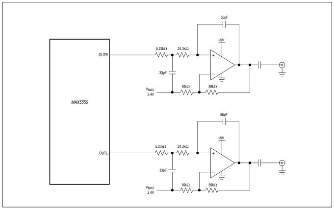
Figure 9. Active Component Analog Output Filter
