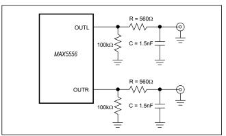
Figure 8. Passive Component Analog Output Filter
