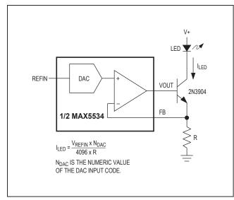
Figure 4. Programmable Current Source Driving an LED
