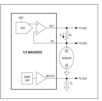
Figure 10. Self-Biased Two-Electrode Potentiostat Application
