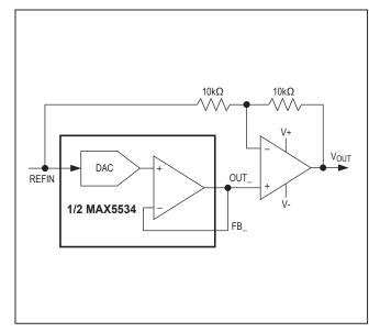
Figure 7. Bipolar Output Circuit
