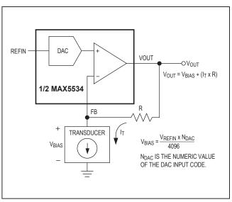
Figure 5. Transimpedance Configuration for a Voltage-Biased Current-Output Transducer
