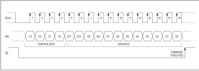
Figure 2. Register Loading Diagram
