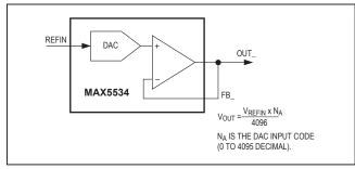
Figure 6. Unipolar Output Circuit
