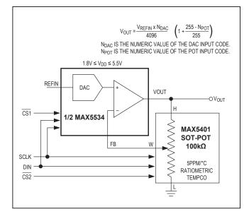
Figure 9. Software-Configurable Output Gain
