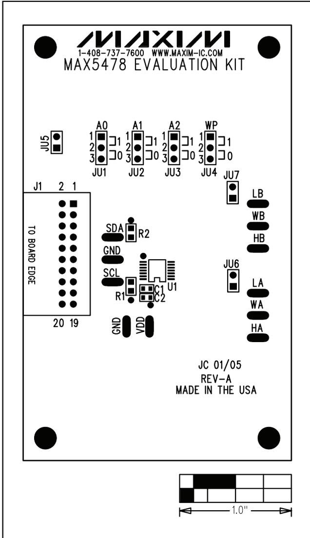
Figure 4. MAX5478 EV Kit Component Placement Guide—Component Side
