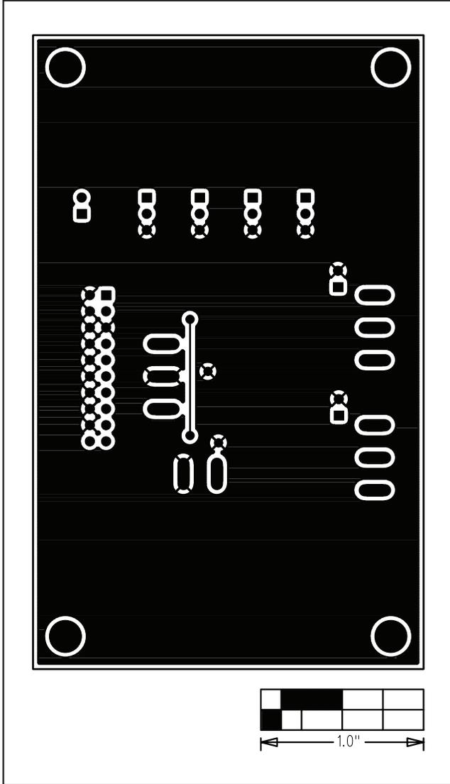
Figure 6. MAX5478 EV Kit PC Board Layout—Solder Side
