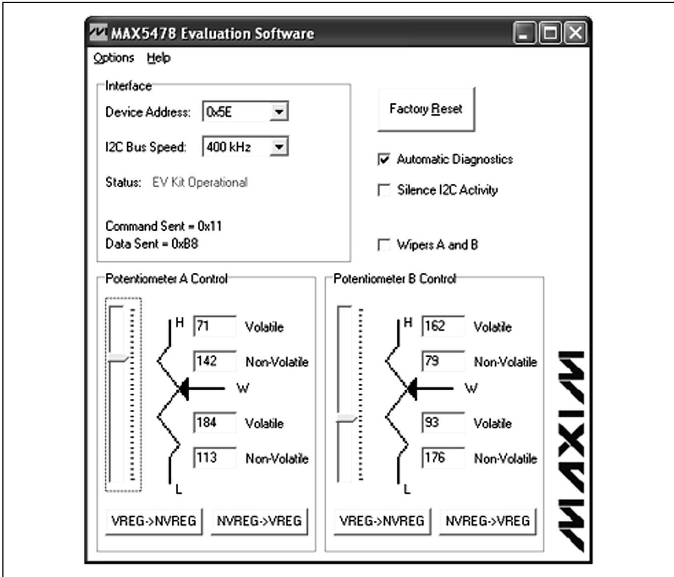
Figure 1. MAX5478 EV Kit Software Main Window
