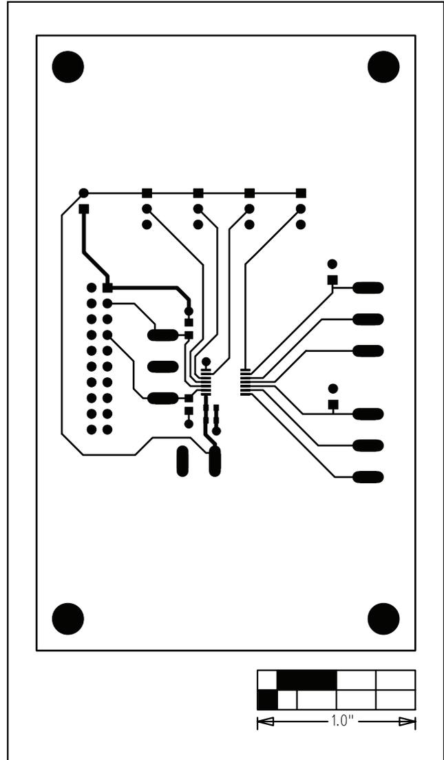
Figure 5. MAX5478 EV Kit PC Board Layout—Component Side
