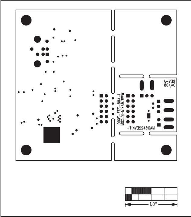
Figure 8. MAX5422 EV Kit Component Placement Guide—Solder Side
