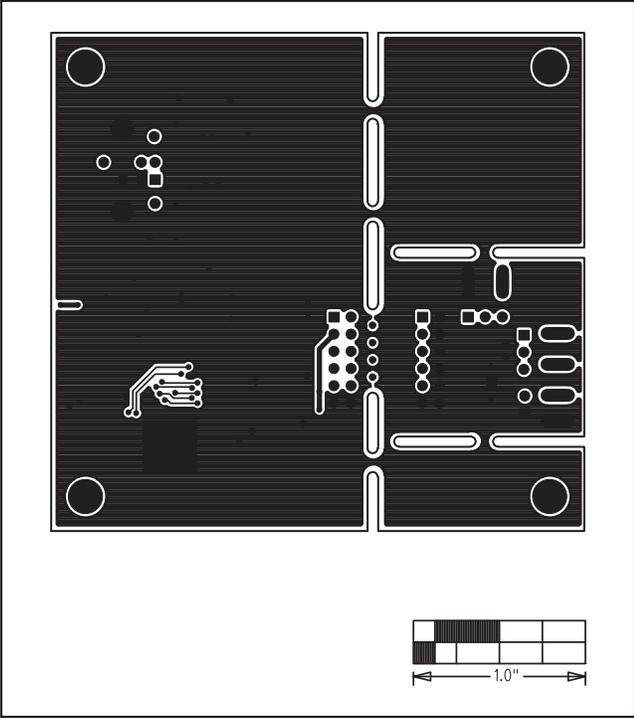
Figure 7. MAX5422 EV Kit PCB Layout—Solder Side
