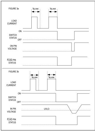
Figure 3. MAX4914B/MAX4915B/MAX4917B Latchoff Fault Blanking
