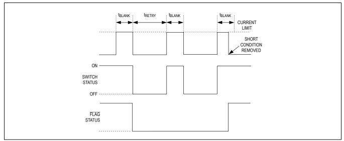
Figure 2. MAX4915A/MAX4917A Autoretry Fault-Blanking Diagram
