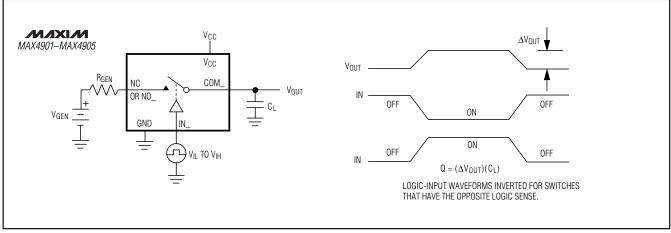
Figure 3. Charge Injection
