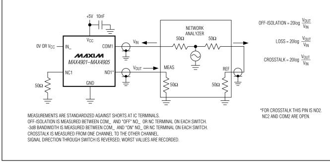
Figure 4. -3dB Bandwidth, Off-Isolation, and Crosstalk
