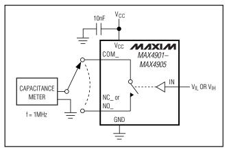
Figure 5. Channel Off-/On-Capacitance
