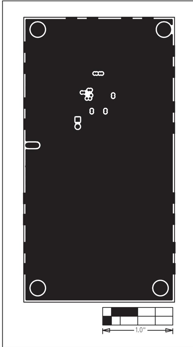
Figure 6. MAX4889A EV Kit PCB Layout—Solder Side
