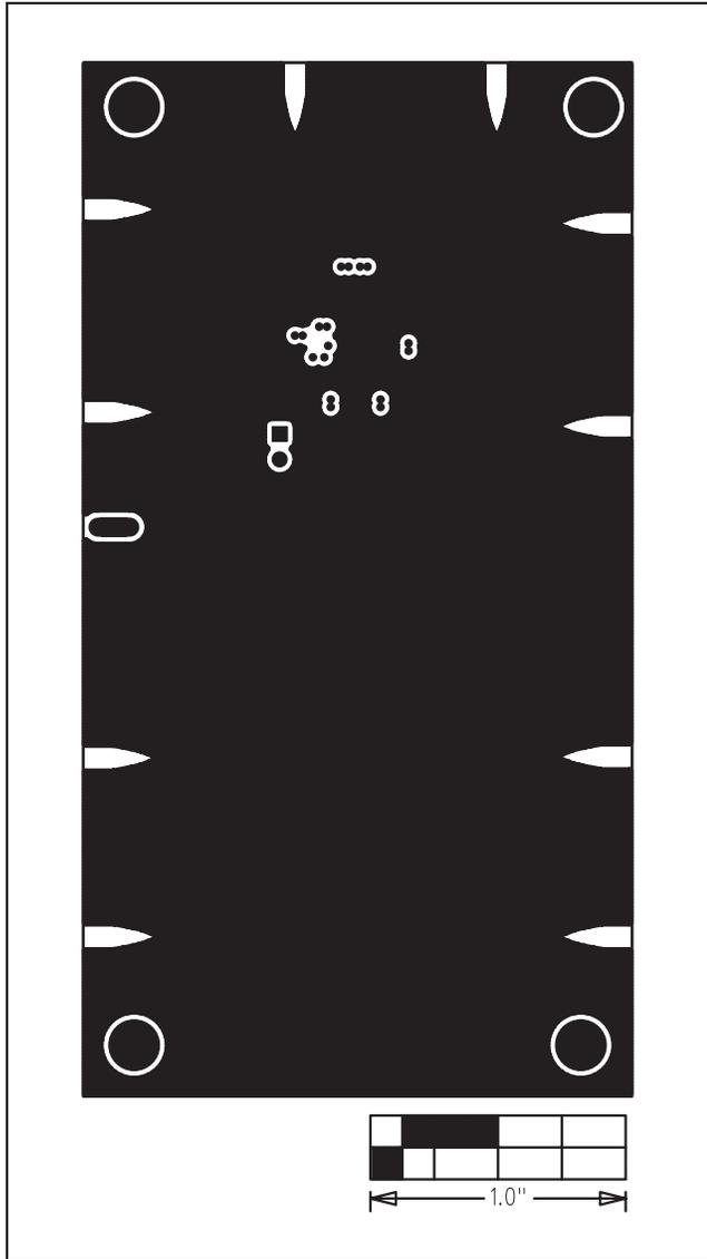
Figure 4. MAX4889A EV Kit PCB Layout—Inner Layer 2
