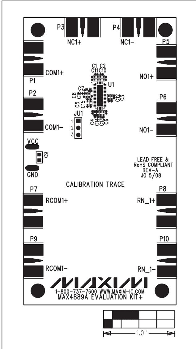
Figure 2. MAX4889A EV Kit Component Placement Guide—Component Side
