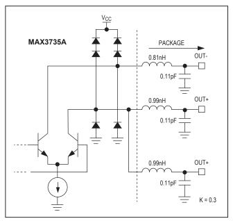
Figure 6. Simplified Output Structure
