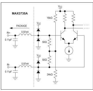
Figure 5. Simplified Input Structure
