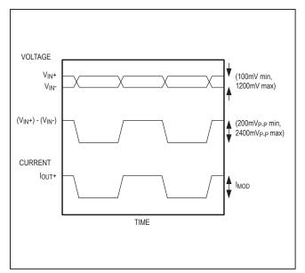
Figure 1. Required Input Signal and Output Polarity
