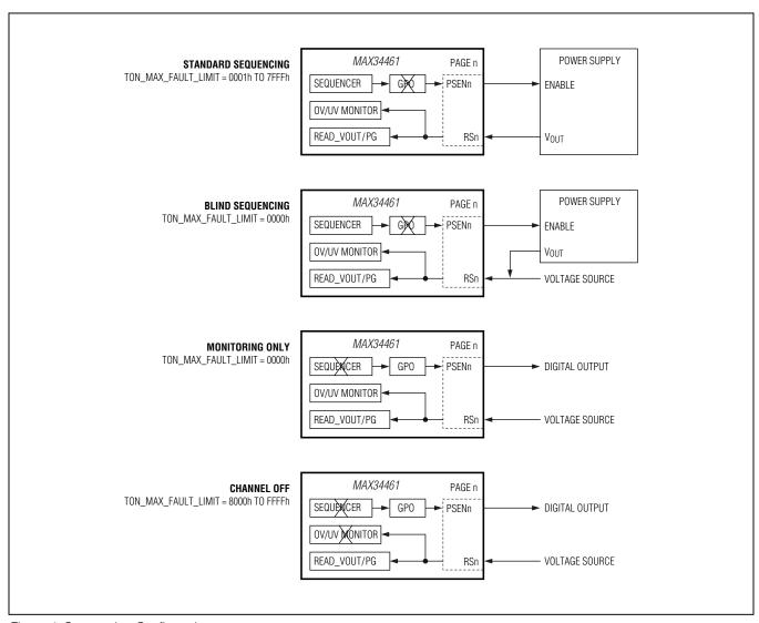
Figure 4. Sequencing Configurations
