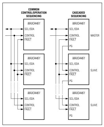
Figure 3. Multiple Device Hardware Connections
