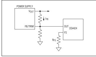
Figure 8. DAC Margining Circuit
