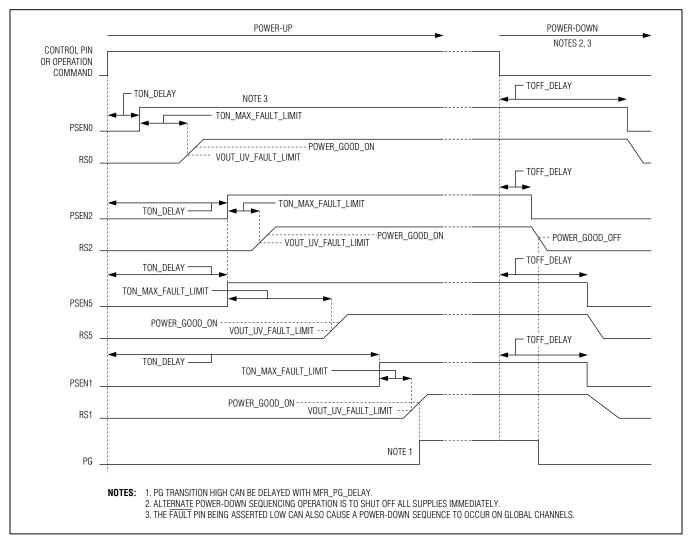
Figure 1. PMBus-Defined Time-Based Sequencing Example
