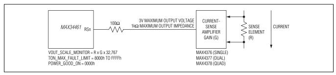
Figure 9. Current-Measuring Circuit
