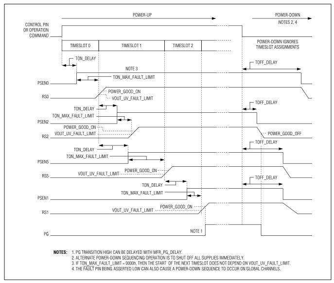
Figure 2. Timeslot-Defined Event-Based Sequencing Example
