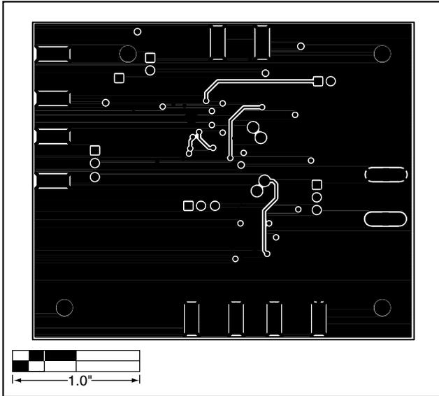
Figure 5. MAX3287 EV Kit PC Board Layout—Solder Side
