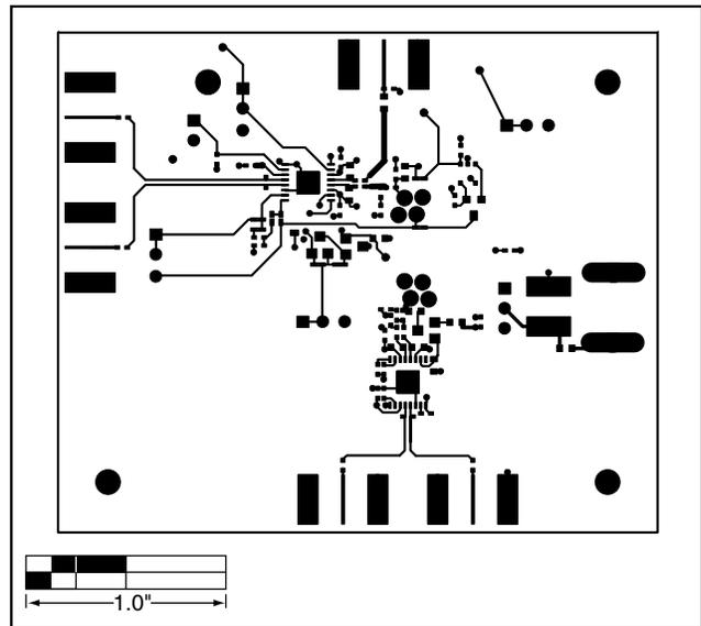
Figure 4. MAX3287 EV Kit PC Board Layout—Component Side
