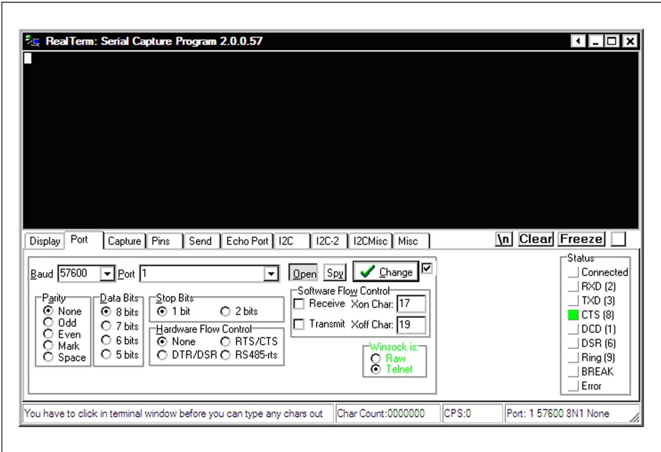
Figure 1. RealTerm Software Main Window (Port Tab)
