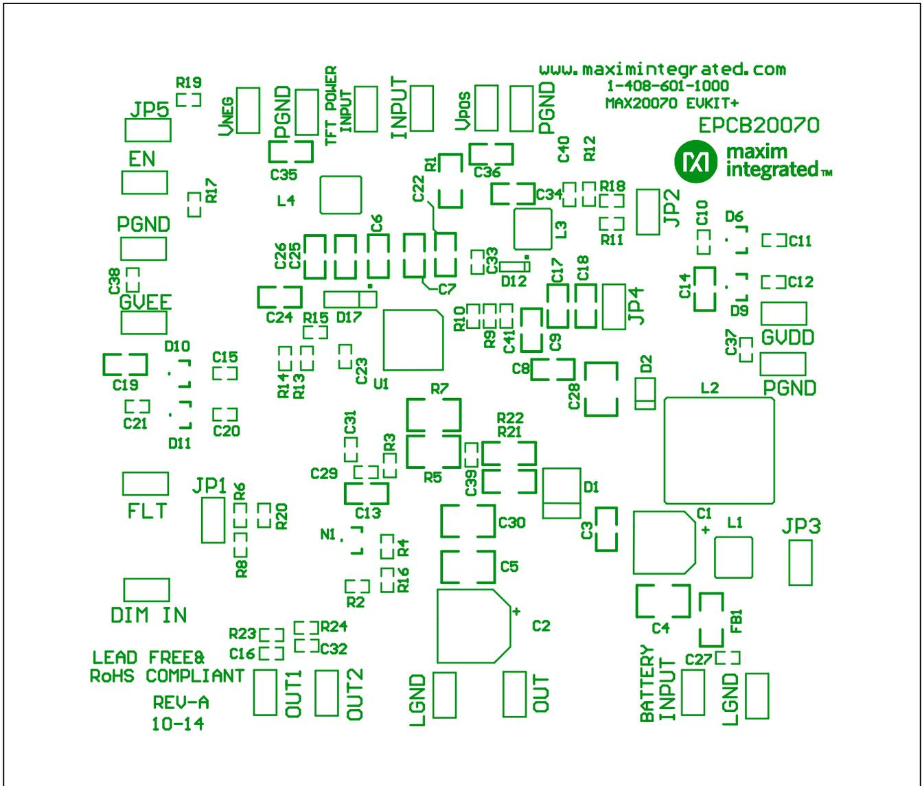
Figure 2. MAX20070 EV Kit Component Placement Guide—Component Side
