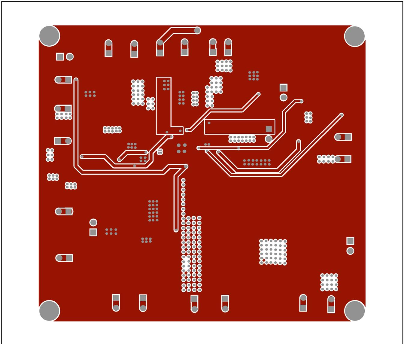
Figure 6. MAX20070 EV Kit PCB Layout—Solder Side
