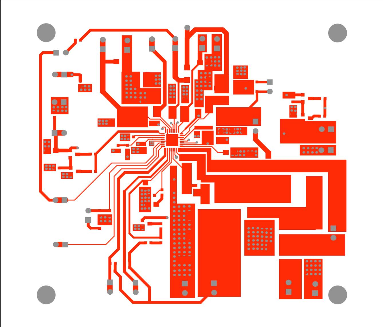
Figure 3. MAX20070 EV Kit PCB Layout—Component Side
