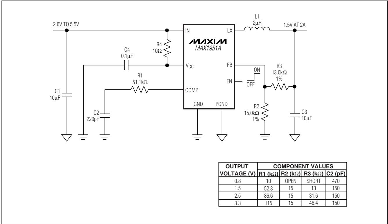
Figure 2. MAX1951A Adjustable Output Typical Application Circuit
