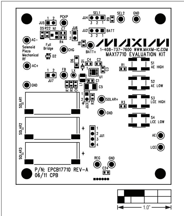
Figure 3. MAX17710 EV Kit Component Placement Guide—Component Side
