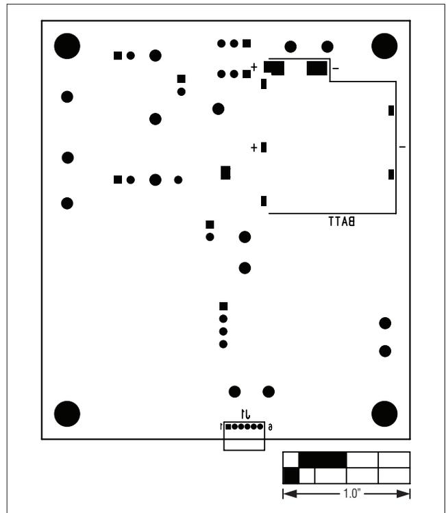
Figure 6. MAX17710 EV Kit Component Placement Guide—Solder Side
