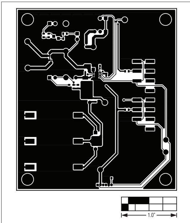
Figure 4. MAX17710 EV Kit PCB Layout—Component Side
