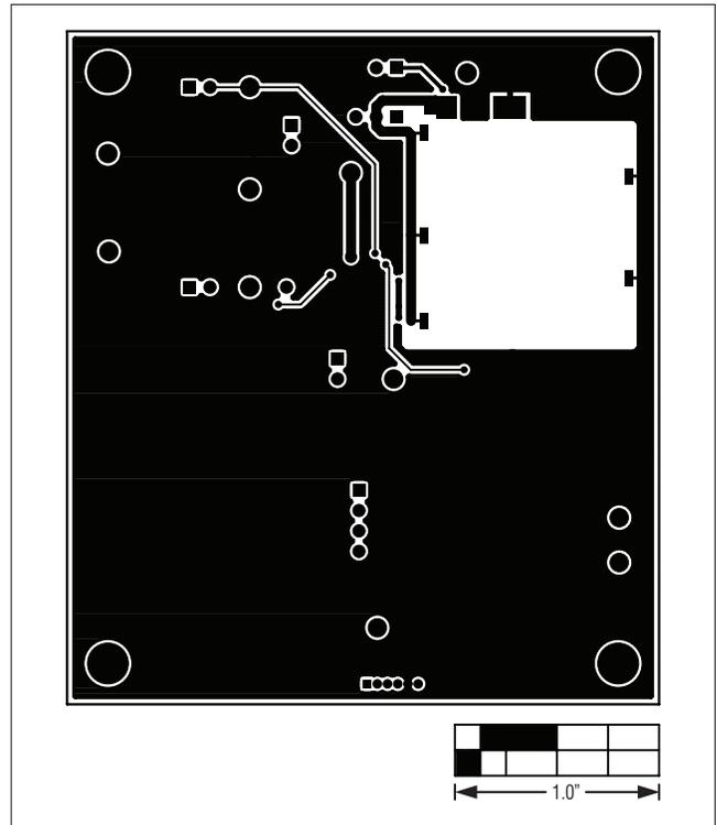
Figure 5. MAX17710 EV Kit PCB Layout—Solder Side
