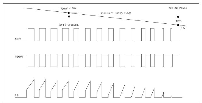
Figure 6. Duty Cycle or Current Soft-Stop
