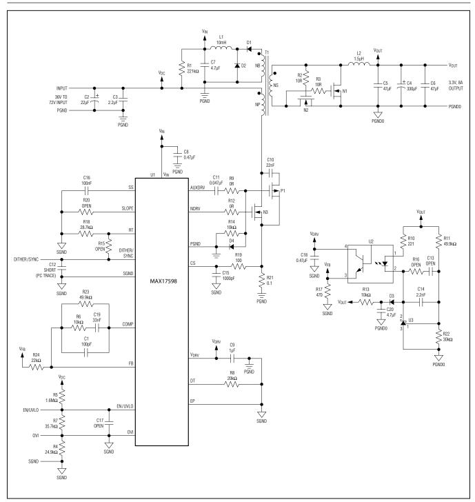
Figure 9. Typical Application Circuit (Telecom Power Supplies)
