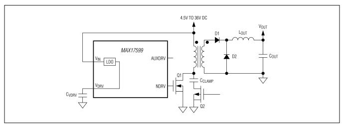
Figure 4. Typical Startup Circuit with IN Connected Directly to DC Input
