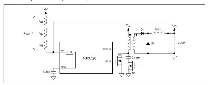
Figure 3. RC-Based Startup Circuit
