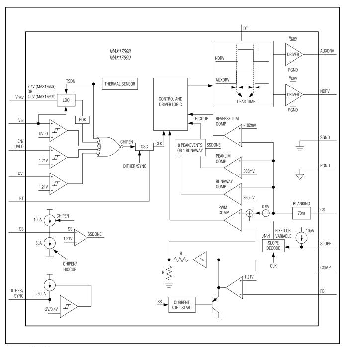
Figure 1. Block Diagram
