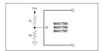
Figure 7. Programming Output Voltage
