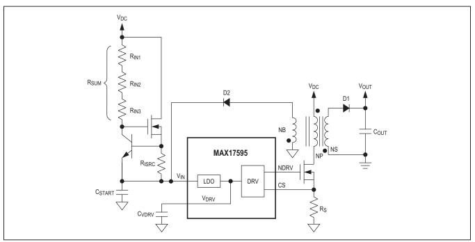
Figure 4. MAX17595 Current-Source-Based Startup Circuit
