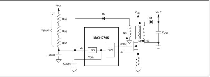
Figure 3. MAX17595 RC-Based Startup Circuit
