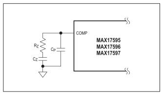
Figure 8. Error-Amplifier Compensation Network
