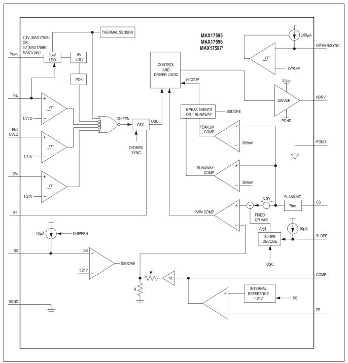
Figure 1. MAX17595/MAX17596/MAX17597 Block Diagram (\*See Note 4.)
