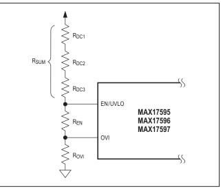
Figure 2. Programming EN/UVLO and OVI
