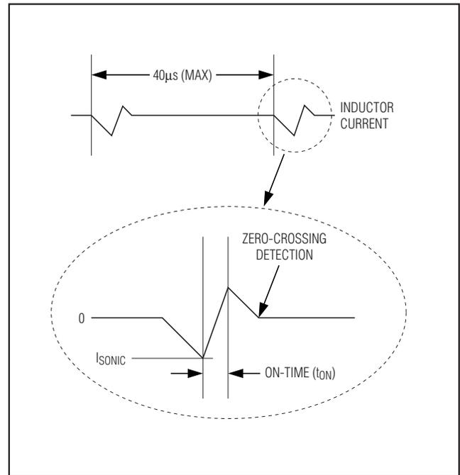
Figure 4. Ultrasonic Waveforms
