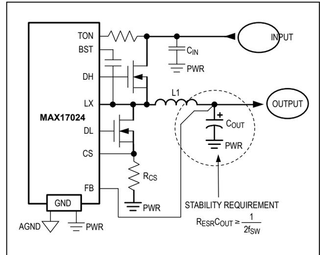
Figure 6. Standard Application with Output Polymer or Tantalum
