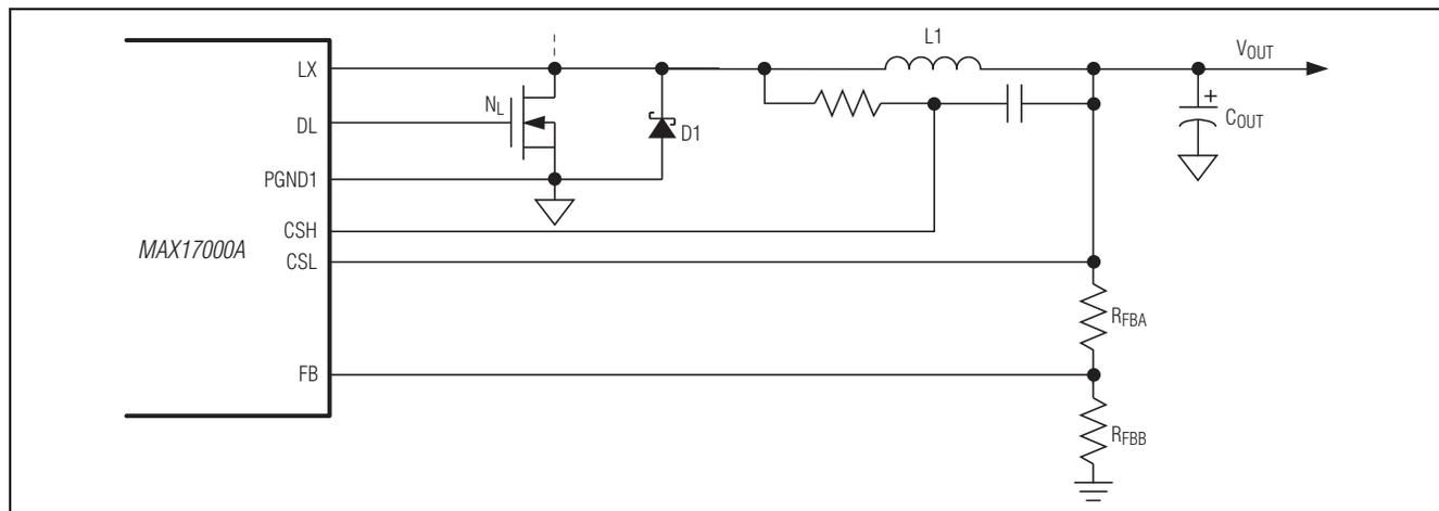
Figure 8. Setting  $V_{\text{OUT}}$  with a Resistive Voltage-Divider
