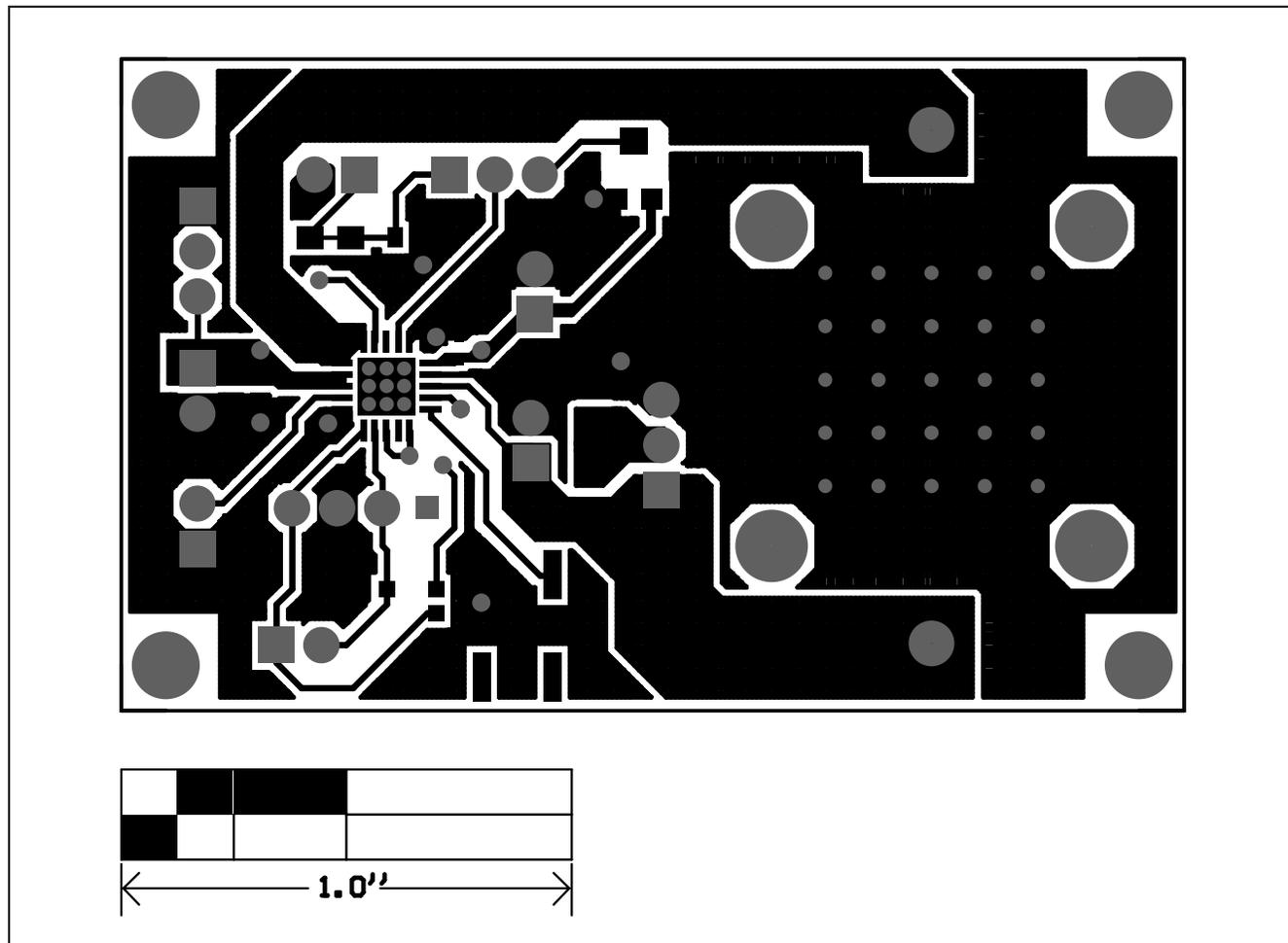
Figure 6. MAX16806 EV Kit PCB Layout—Component Side
