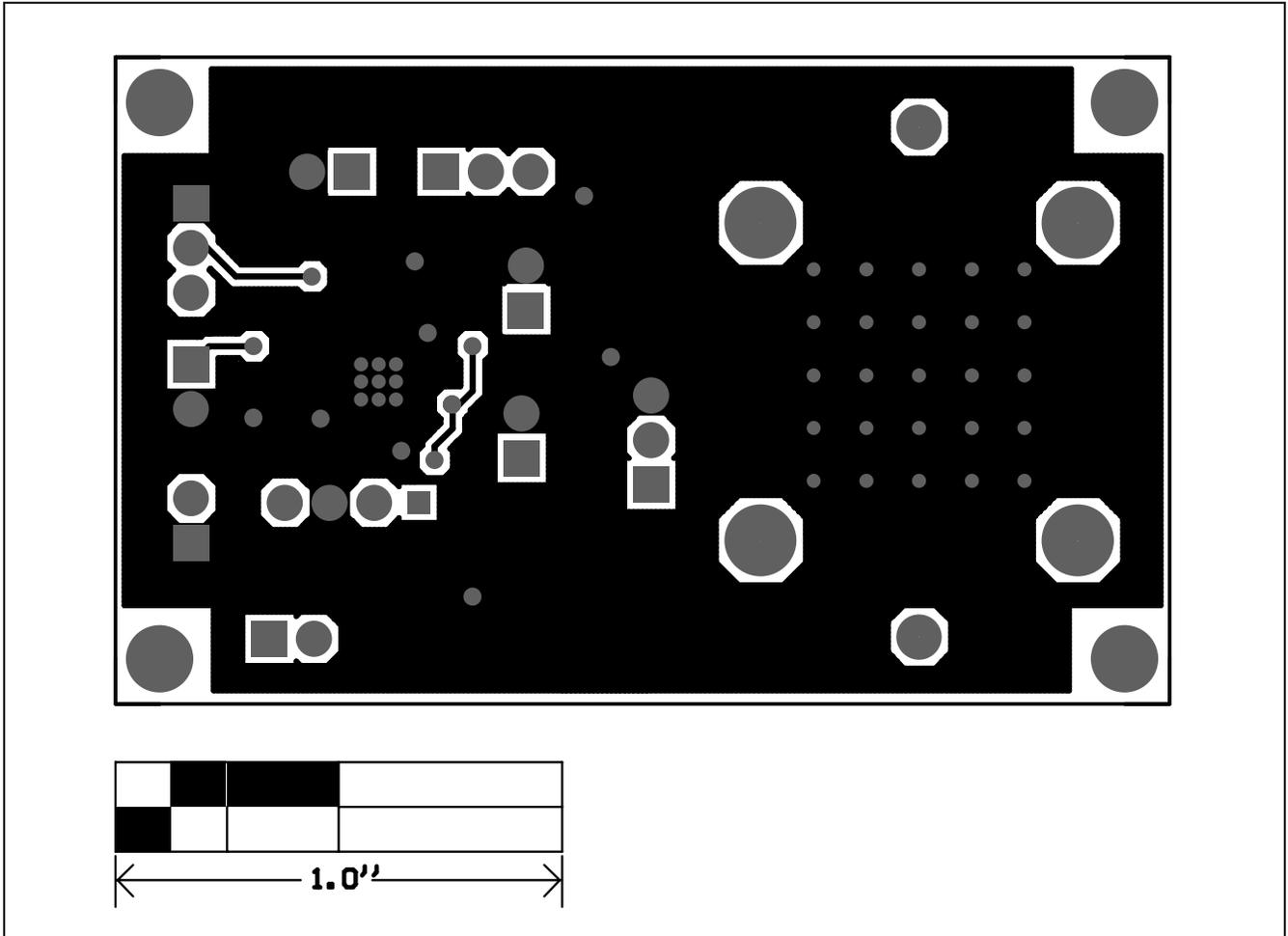
Figure 7. MAX16806 EV Kit PCB Layout—Solder Side
