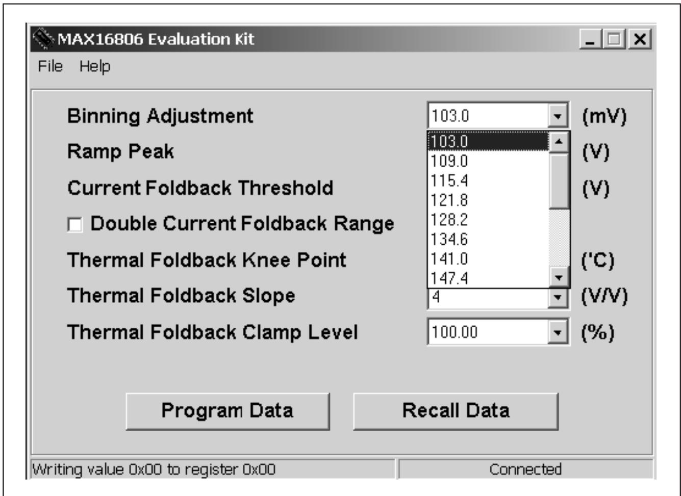
Figure 3. MAX16806 EV Kit Software—Writing to Dynamic Registers
