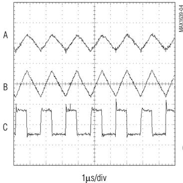
$V_{IN} = 5\text{V}$ ,  $V_{OUT} = 2.5\text{V}$ ,  $\text{LOAD} = 0\text{A}$
