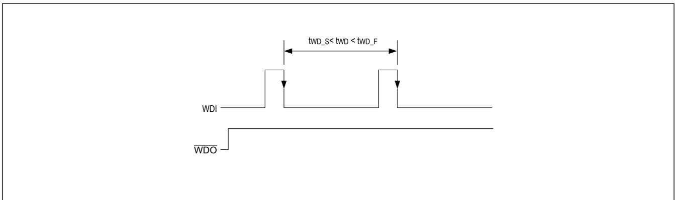
Figure 5. Normal Watchdog Operation (No Watchdog Output Pulse)
