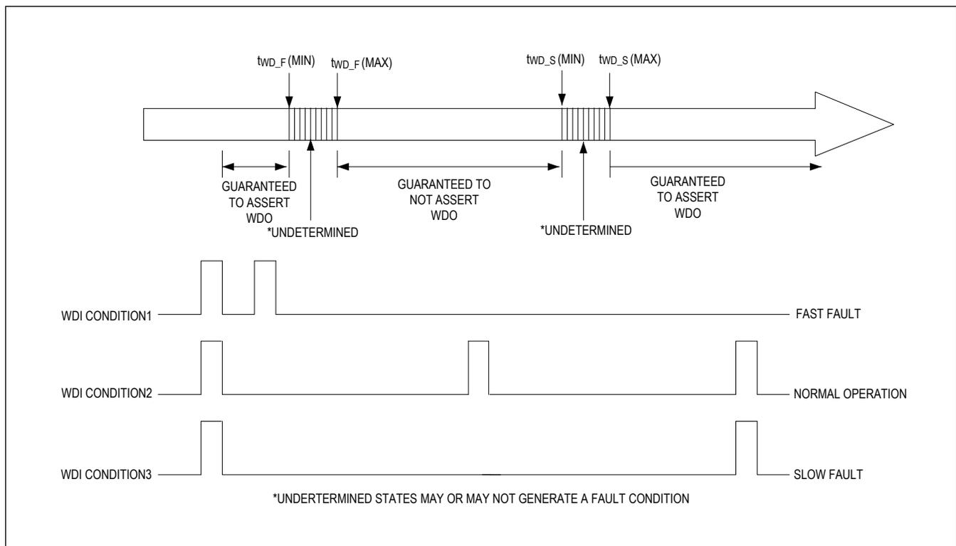
Figure 1. MAX16136 Detailed Watchdog Input Timing Relationship
