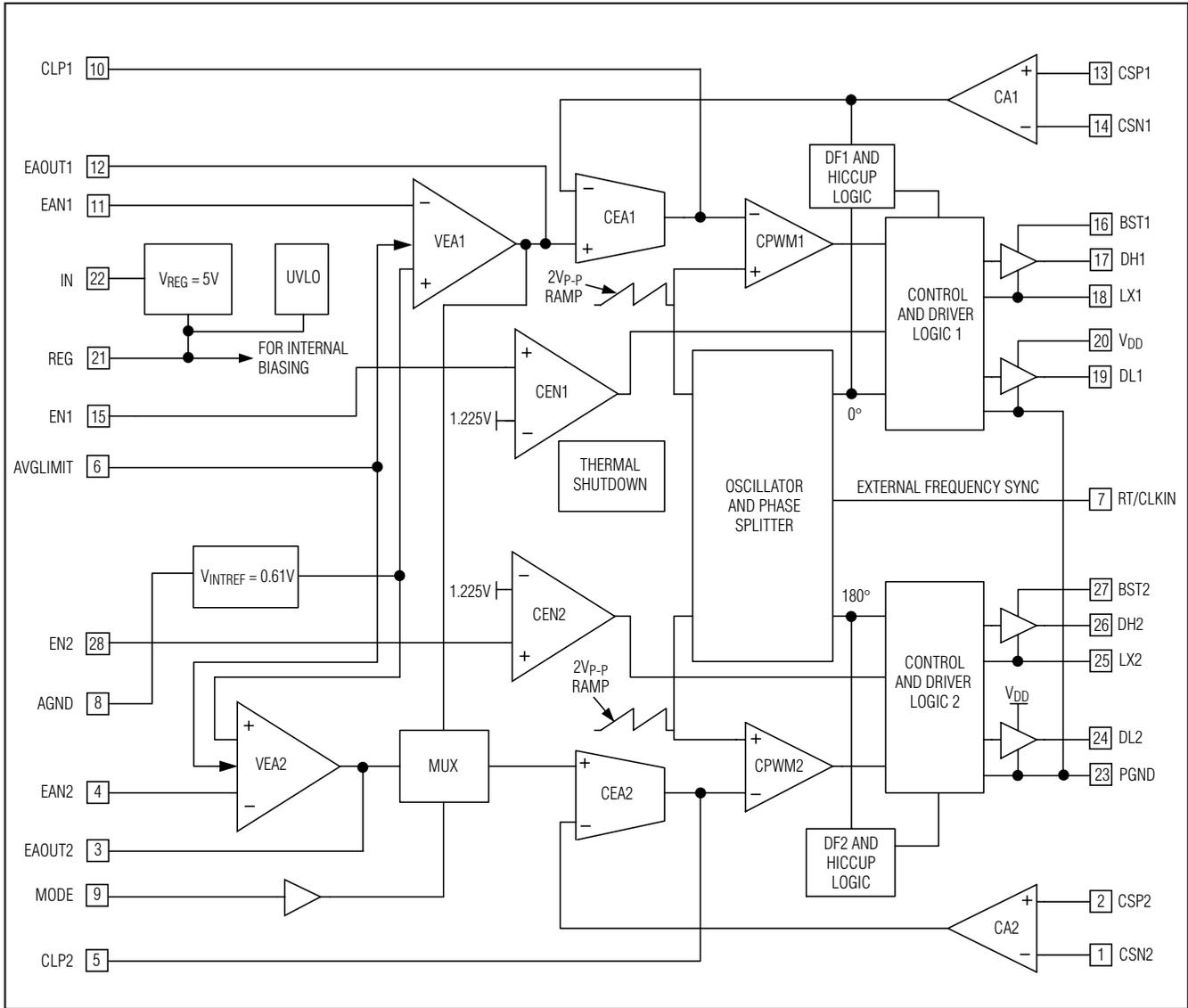
Figure 1. Block Diagram
