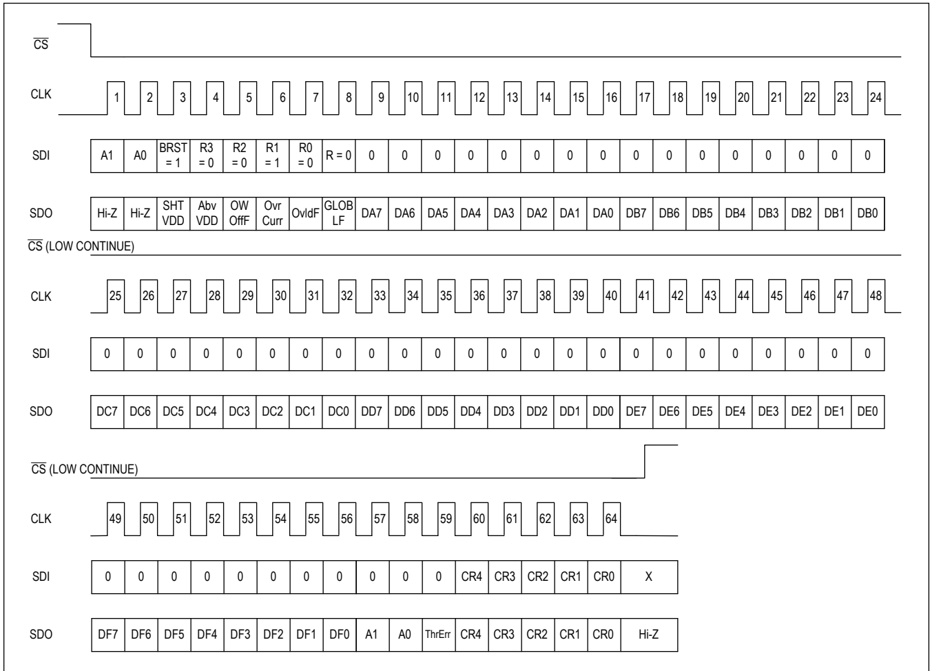
Figure 15. SPI Burst Read with CRC Enabled
