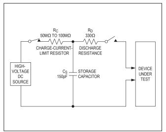
Figure 6. IEC 61000-4-2 ESD Test Model
