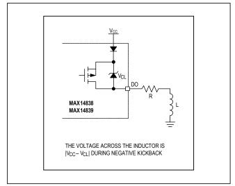
Figure 2. High-Side Mode with Ground-Connected Load
