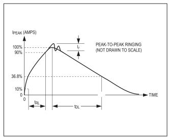
Figure 5. Human Body Current Waveform
