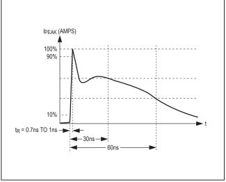
Figure 7. IEC 61000-4-2 ESD Generator Current Waveform
