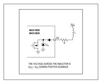
Figure 3. Low-Side Mode with Supply-Connected Load
