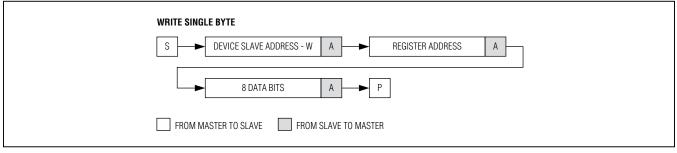
Figure 8. Write-Byte Sequence
