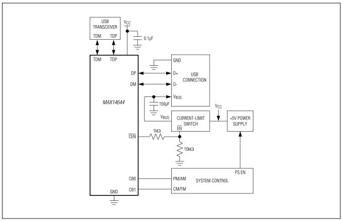
Figure 5. MAX14644 Peripheral Reset Applications Diagram
