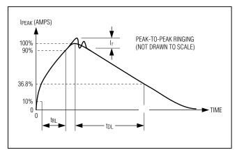
Figure 14. Human Body Current Waveform
