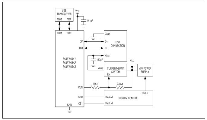
Figure 6. MAX14641/MAX14642/MAX14643 Peripheral Reset Applications
