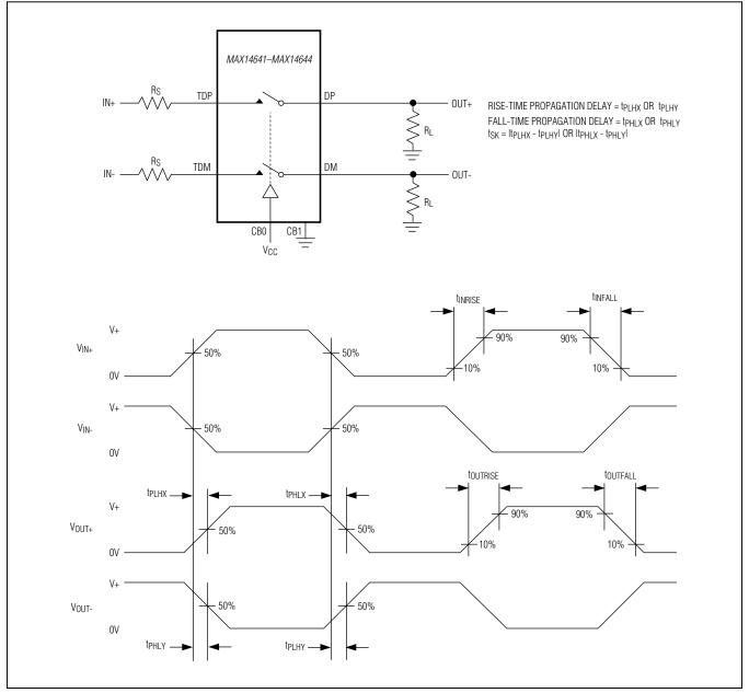
Figure 2. Propagation Delay and Output Skew
