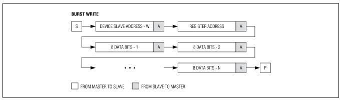
Figure 9. Burst Write Sequence
