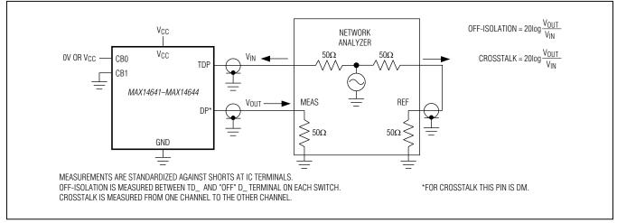
Figure 3. Bandwidth, Off-Isolation, and Crosstalk
