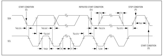
Figure 4. I<sup>2</sup>C Timing Diagram. Note that  $t_R$  and  $t_F$  are per the I<sup>2</sup>C fast-mode specification.
