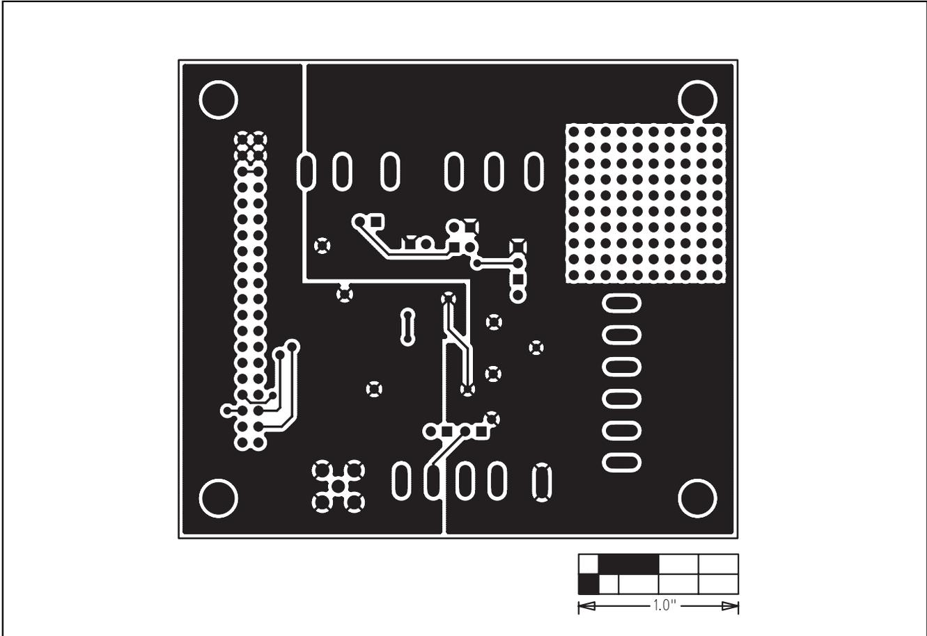
Figure 4. MAX1402 EV Kit PCB Layout—Solder Side
