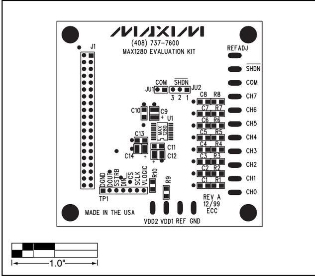
Figure 2. MAX1280 EV Kit Component Placement Guide—Component Side
