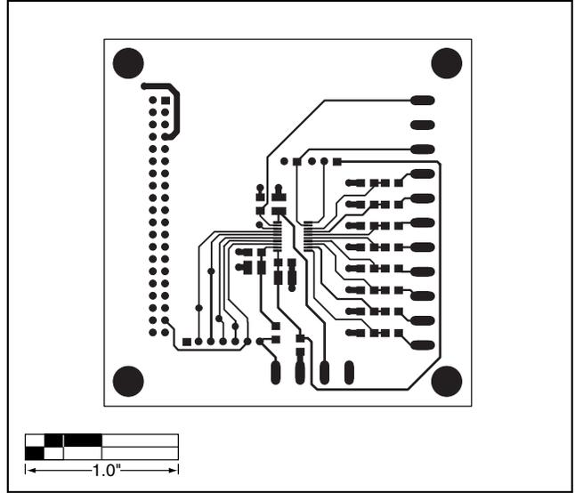
Figure 3. MAX1280 EV Kit PCB Layout—Component Side
