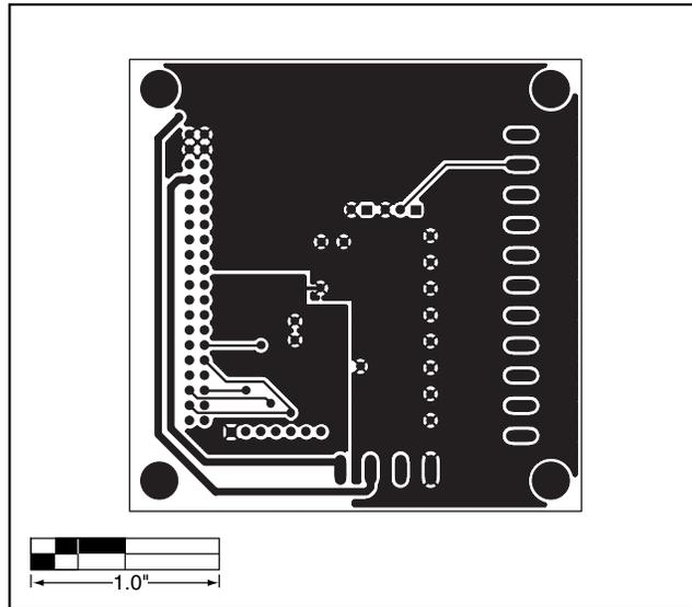
Figure 4. MAX1280 EV Kit PCB Layout—Solder Side
