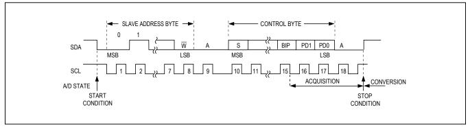
Figure 9. Complete 2-Wire Serial Write Transmission
