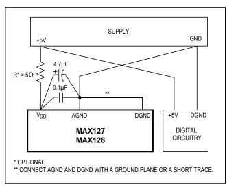
Figure 14. Power-Supply Grounding Connection
