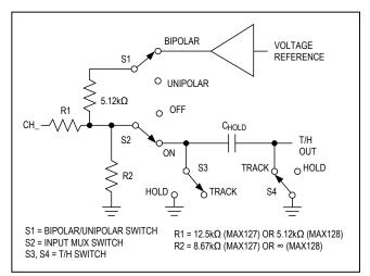
Figure 2. Equivalent Input Circuit
