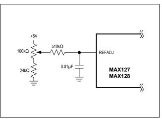
Figure 12. Reference-Adjust Circuit
