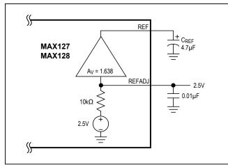
Figure 11c. External Reference, Reference at REFADJ
