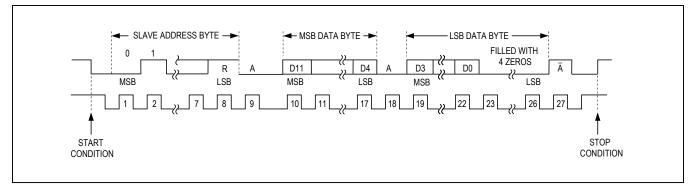
Figure 10. Complete 2-Wire Serial Read Transmission
