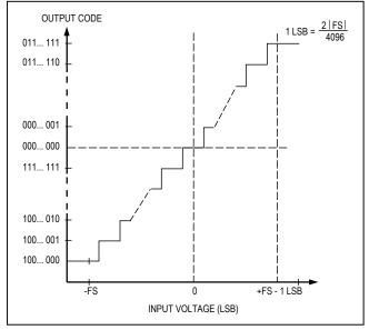
Figure 13b. Bipolar Transfer Function
