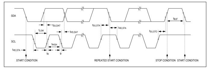
Figure 5. 2-Wire Serial-Interface Timing Diagram
