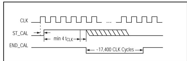
Figure 8. Timing for Start and End of Calibration
