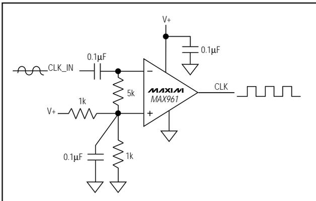
Figure 6. Clock Generation Circuit Using a Low-Noise Comparator
