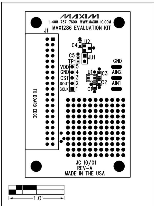
Figure 3. MAX1286 EV Kit Component Placement Guide—Component Side
