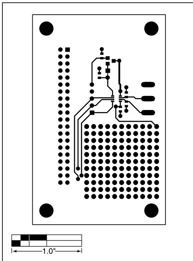
Figure 4. MAX1286 EV Kit PC Board Layout—Component Side
