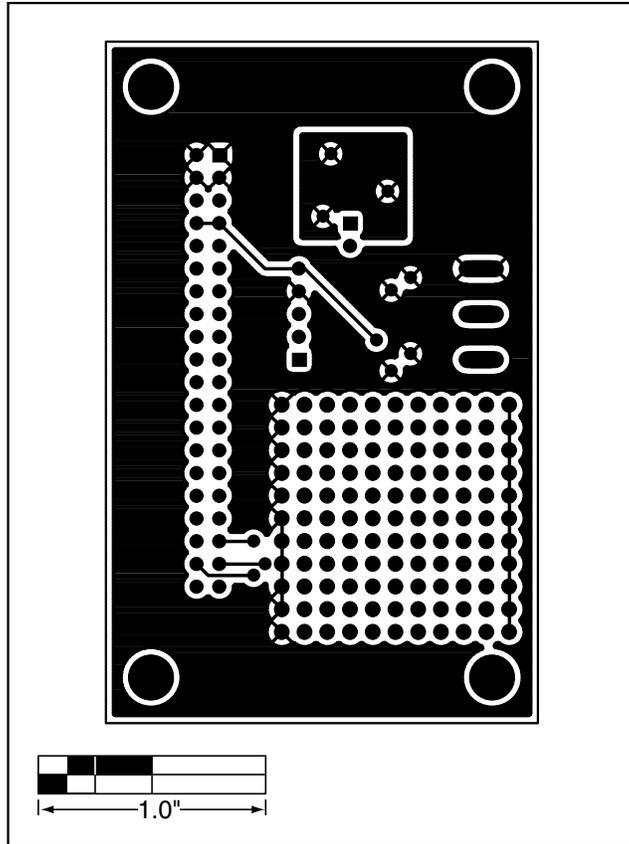
Figure 5. MAX1286 EV Kit PC Board Layout—Solder Side
