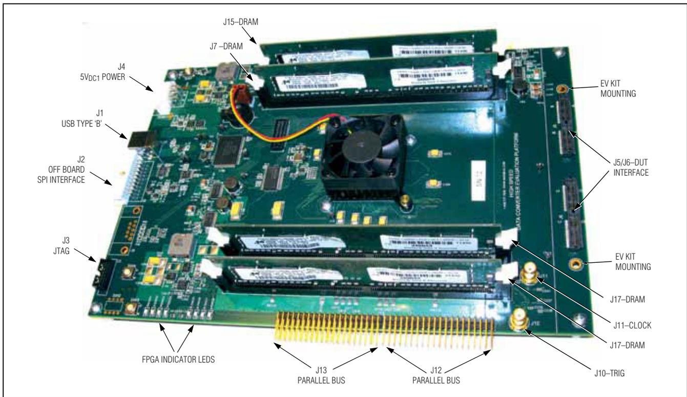
Figure 2. High-Speed Data Converter Evaluation Platform (PCB Photo)
