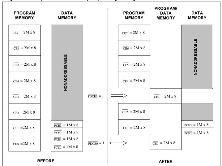
Figure 1. Example External Memory Map—Merged Program/Data
