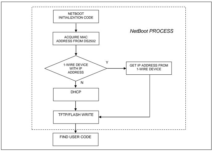
Next, the DS80C400 ROM searches the 1-Wire bus for an external device (separate from the device containing the MAC address) that contains an IP address and TFTP server IP address. In order to correctly acquire the IP and TFTP server addresses from an external 1-Wire device, the data read from the device must conform to a specific format. This format is shown in Figure 15.
