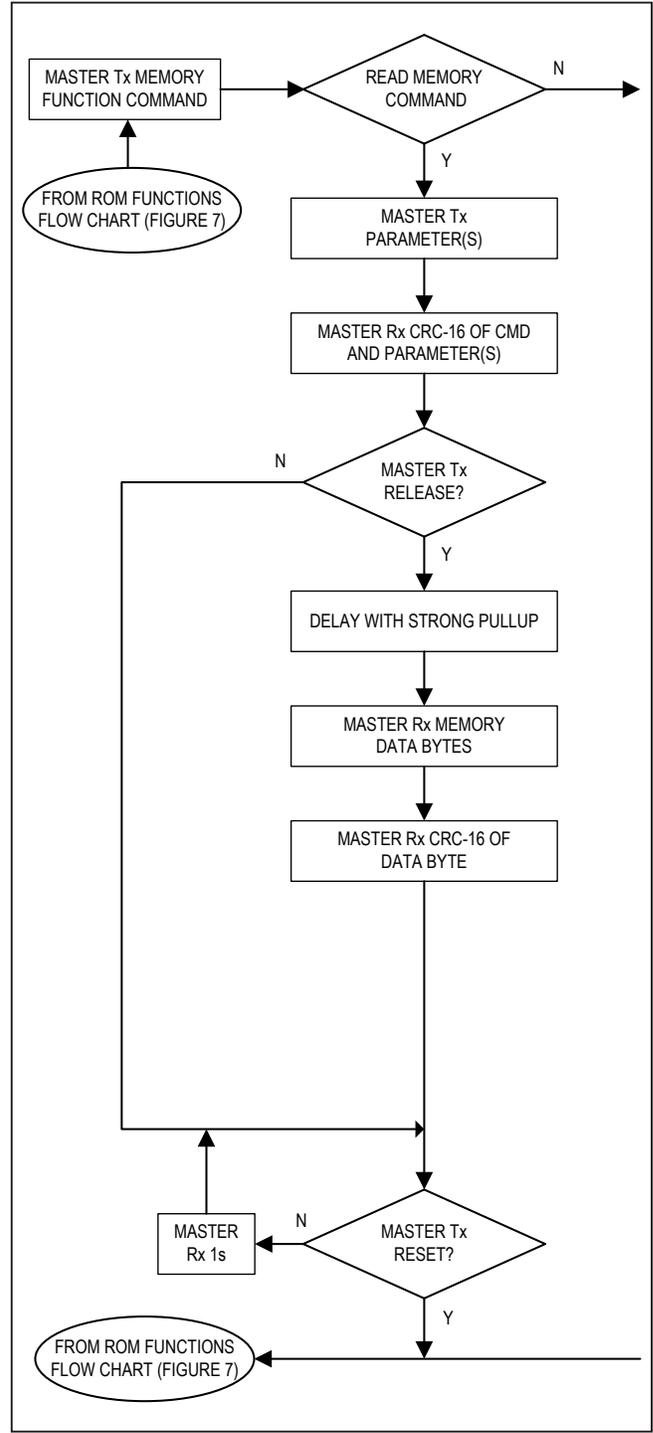
Figure 3. 1-Wire Device Data Read Flow Chart
