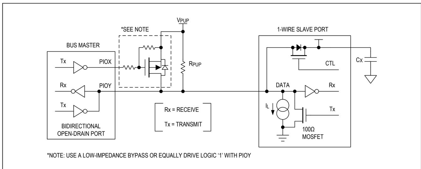
Figure 4. Hardware Configuration
