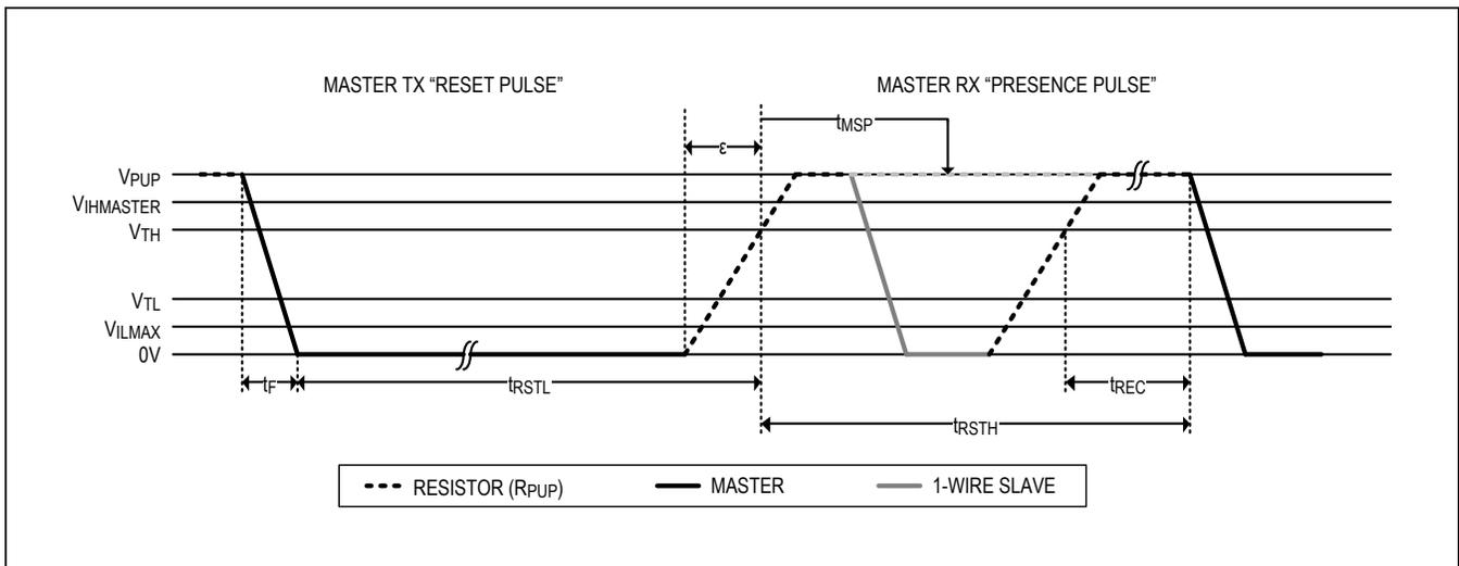
Figure 5. Initialization Procedure: Reset and Presence Pulse
